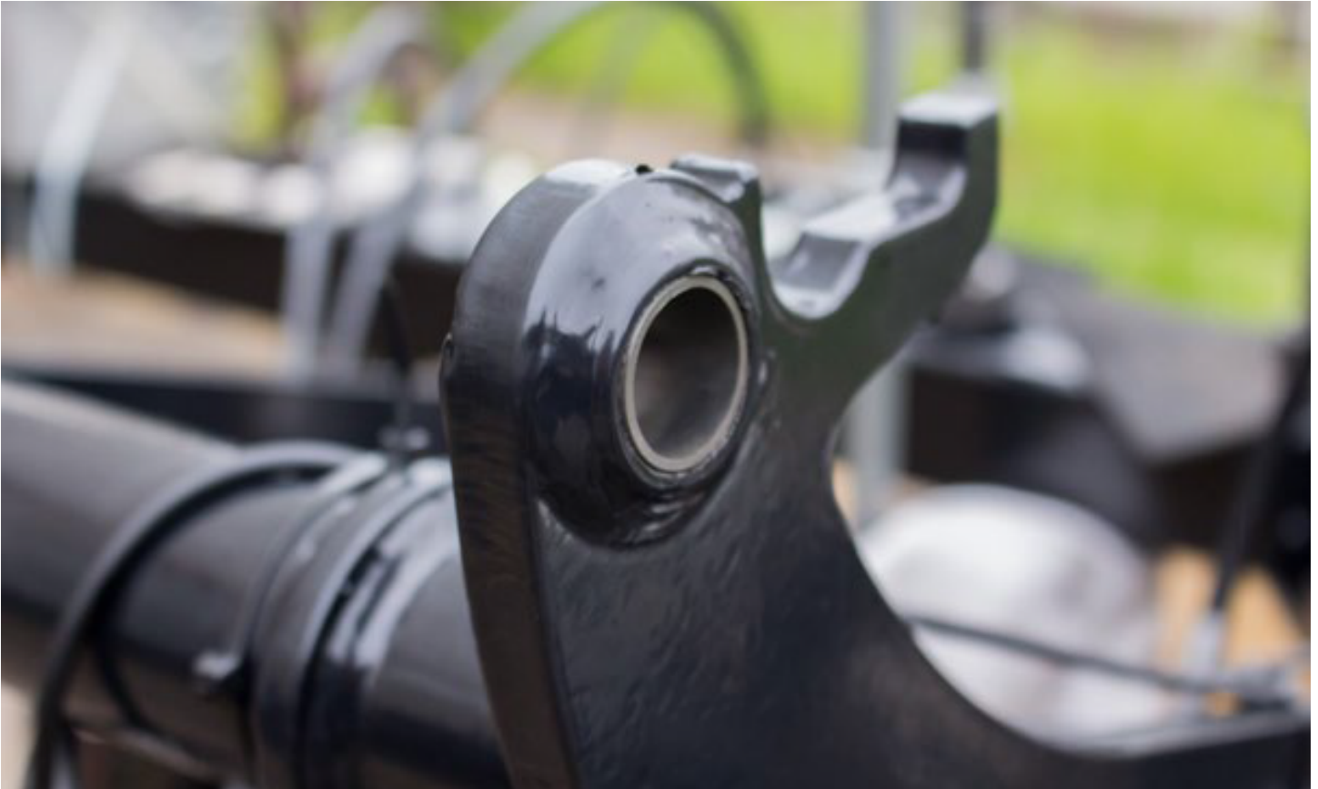
Bearing position with pressed-in plastic plain bearing
