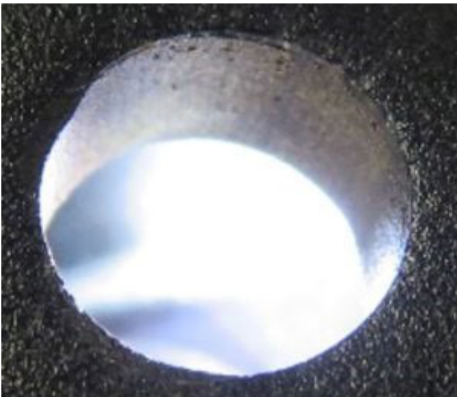
Housing bore with burr (top left)
