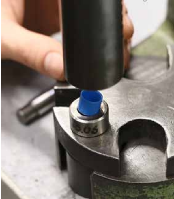
Press-fit in an inserted plastic bushing
