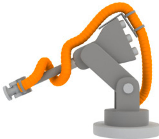
Jointed-arm (six-axis / articulated) robots use two straight components with a rotating shoulder and elbow in horizontal axes.
