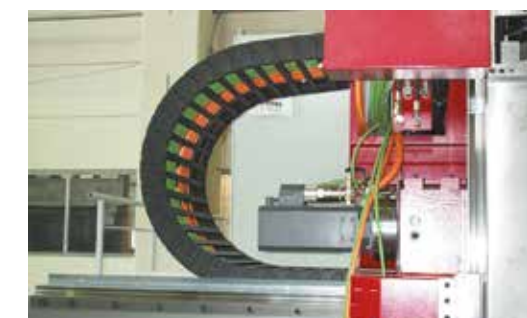
Pre-harnessed igus® energy supply systems for machine tool manufacture. E-Chain®: System E4/4
