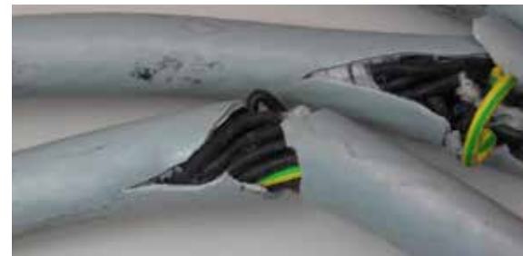
Jacket damage already after 41,000 strokes ...
