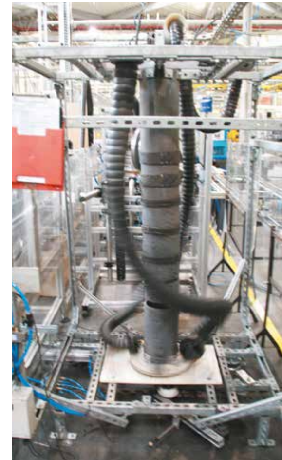
igus® test lab: The cables were tested in movements of \pm 270^\circ
