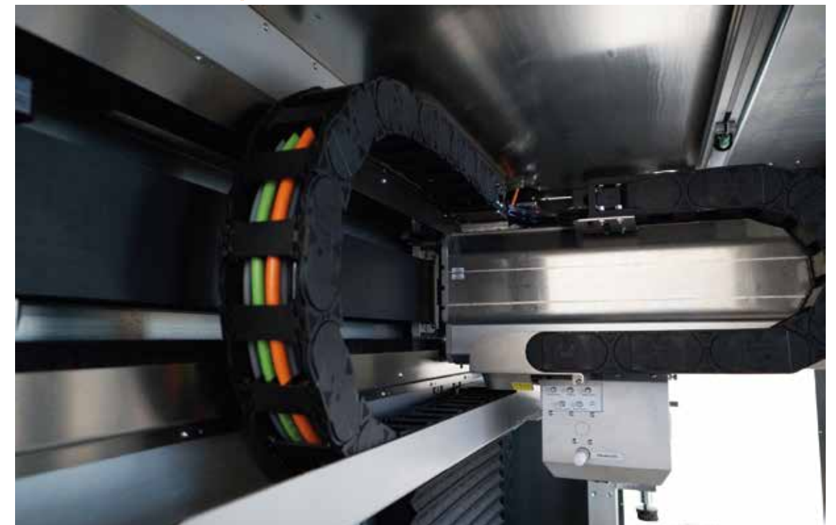
Linear robot with chainflex® servo and measuring system cables, short travel distance
