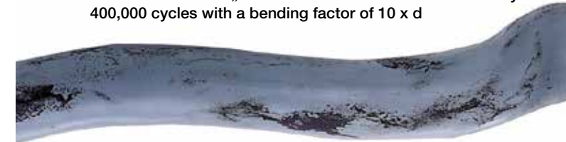
Picture 4: Shielded „chain-suitable“ control cable after only 400,000 cycles with a bending factor of 10 x d
