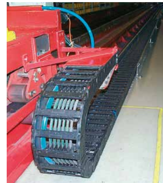
chainflex® CF5/CF6 for storage retrieval unit: Long travel in longitudinal axis. E-Chain®: Series E4/00 with igus® guide trough made of steel
