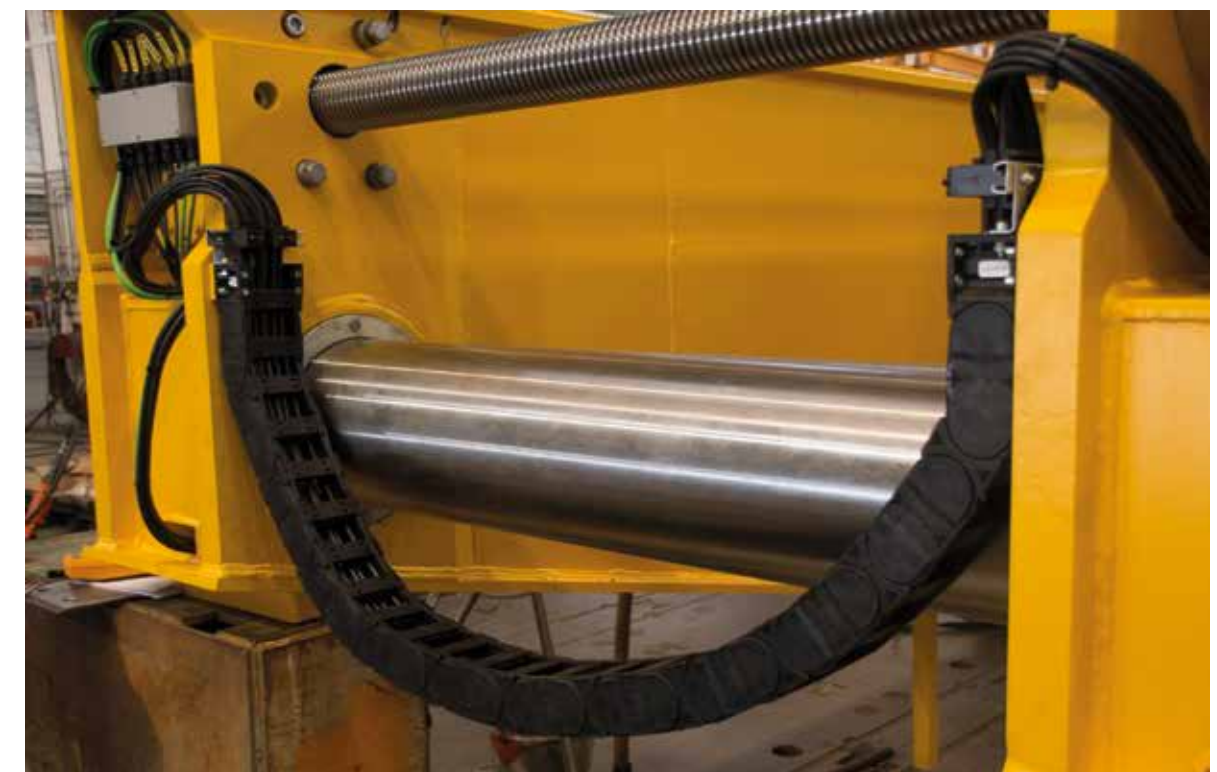
chainflex® CF891 in adjustment device in process crane
