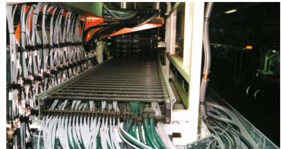
chainflex® CF5 and CF6 control cables (green) as well as CF211 measuring system cables (gray) in a screwing station of a car factory. E-Chain®: System E4/00 with chainfix clip strain relief devices.
