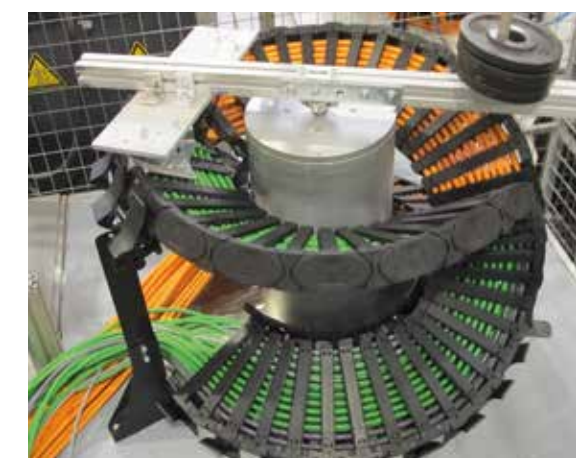
Rotary movement tests: Demanding chain applications with small radii
