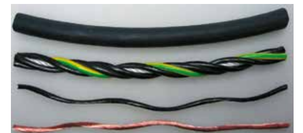
The individual elements of the CF9 from the cable piece dissected for the test setup.
