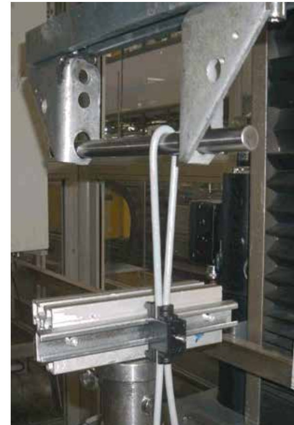
igus® tensile strength test with CFX clamps
