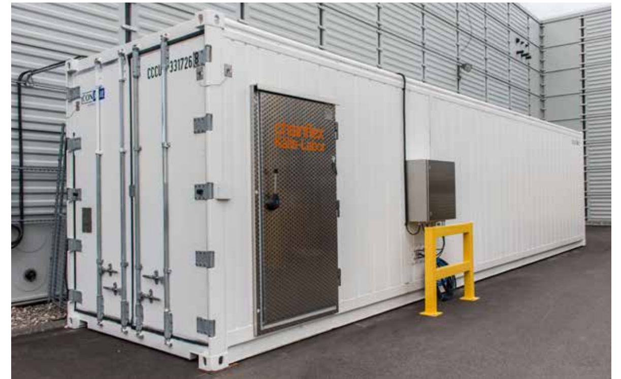
40-foot climatic container for cable tests in continuous motion at -40°F
