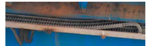
An igus® energy supply system with an approx. length of 85 ft. in a stainless steel trough.
