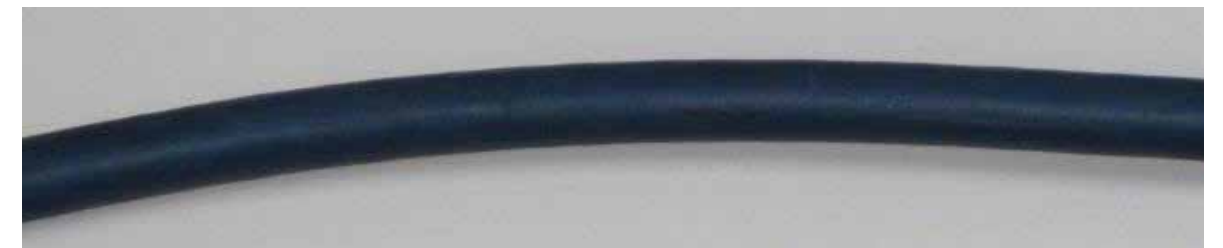
520,000 strokes without any damage, which the CF9-15-18 managed in this test
