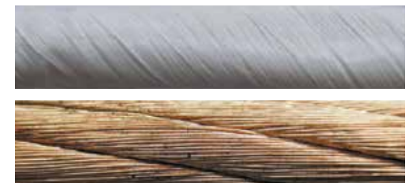
igus® test lab: The cables were tested in movements of \pm 270^\circ
