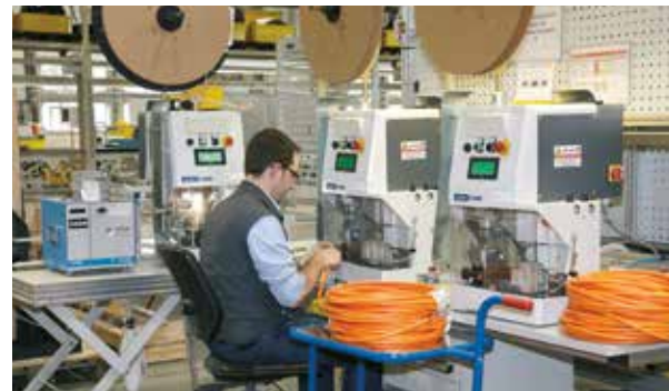
Modern machinery - automatic stripper-crimper
