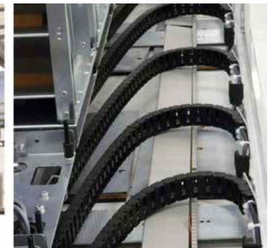
chainflex® cables (e.g. CF211) and igus® e-chains® (E065 series) in a pharmacy picking systems
