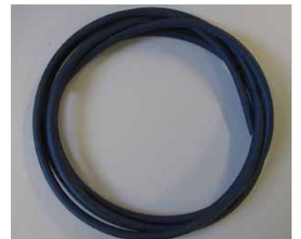
Result chainflex® TPE jacket: Cable after the test with 520,000 strokes
