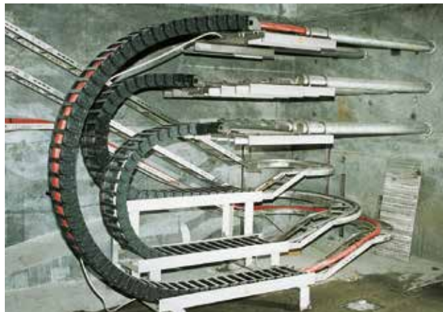
The igus® product range offers up to 12 different bend radii for each chain series from stock. Here series 50 in the Storebaelt bridge project.
