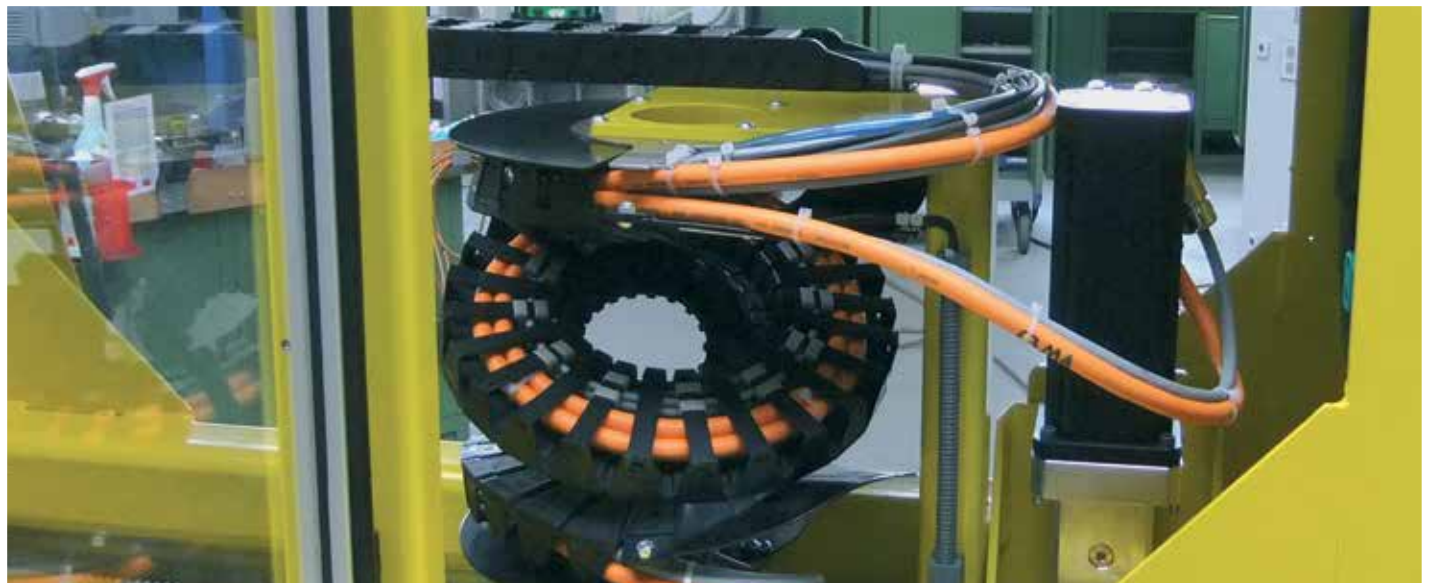
igus® twisterband TB30 for circular movements up to 360°, E2 mini and E2/000 e-chains® are used in this loading and unloading unit
