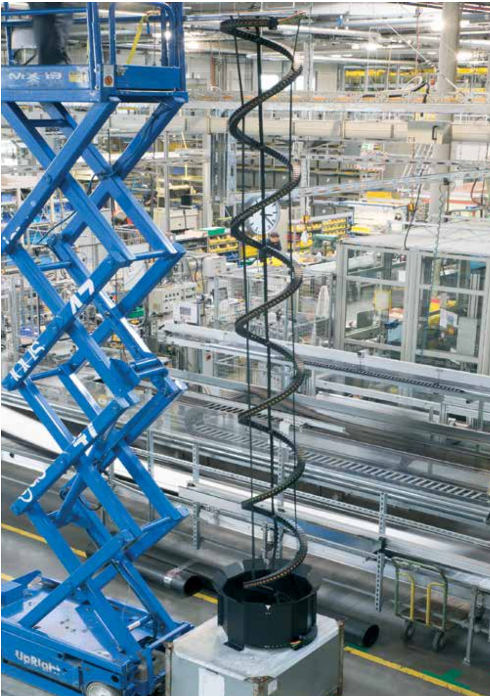
liftband test setup in the igus® test lab
