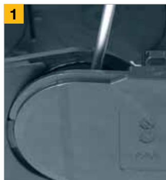
1 Remove crossbars, clips, lids and bottoms at the outer links
