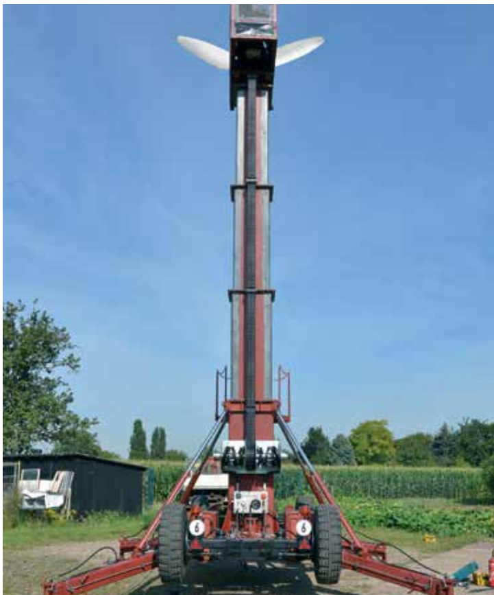
The igus® e-spool in an extendable fan system made by Becker Electric Forklift Service in Ertstadt. Vertically extendable up to 10m. The e-spool supplies the motor with media and energy cables
