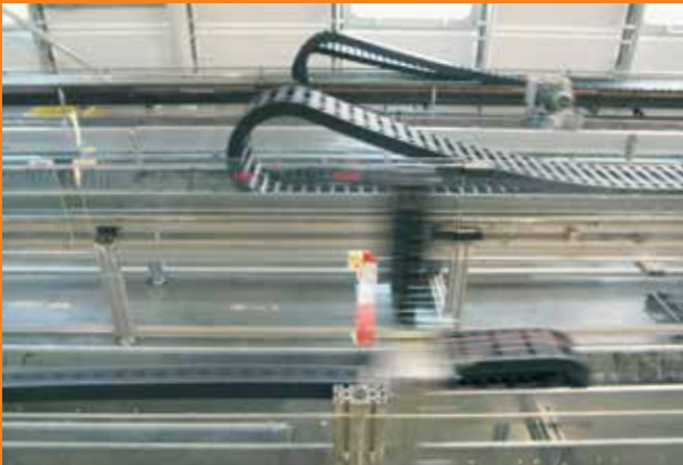
Speeds up to 10m/s, acceleration up to 200m/s 2 are tested
