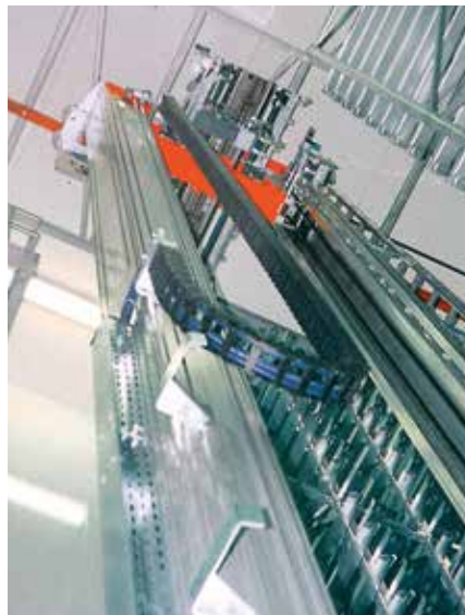
Hanging assembly with one-sided U profile
