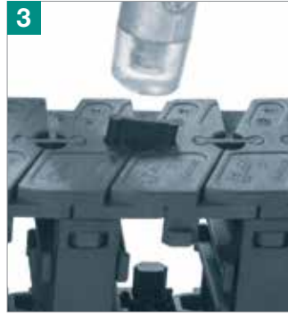
3 Gently insert connector by using a hammer
