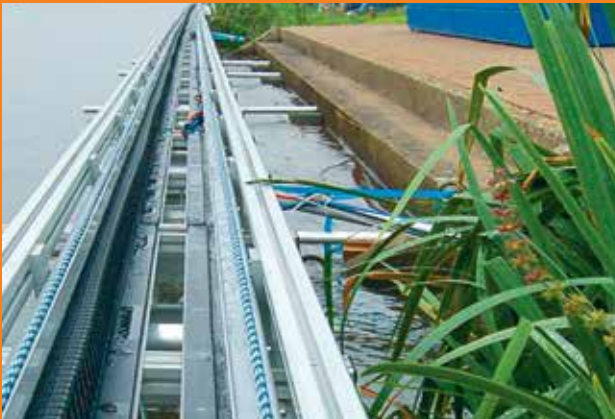
Long travel, side-mounted installation using the vibration-free and low-noise series E6.29 in a camera application
