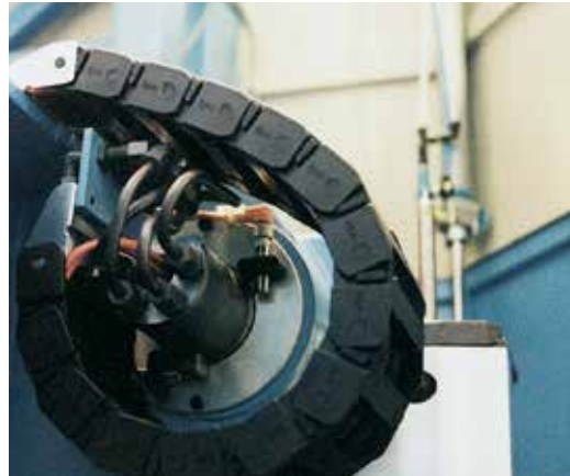
Rotary motion with a standard igus® e-chain®
