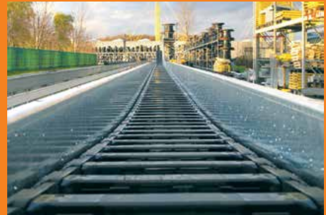
Long travel test facility - 125m travel length, speed 300m/min
