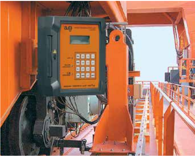
Long travels with electronics Push/Pull-force monitoring with the igus® PPDS System
