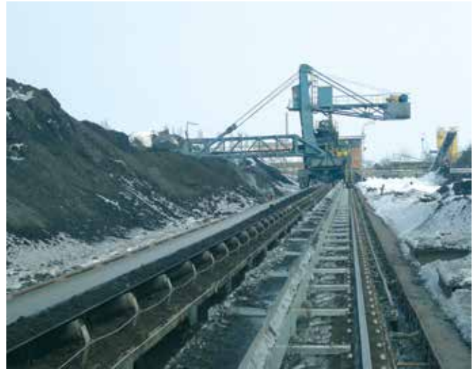
Series 4040HD on (180 m) travel lengths with housing. -40°F/+104°F (-40°C to +40°C) temperature range and high dirt pollution
