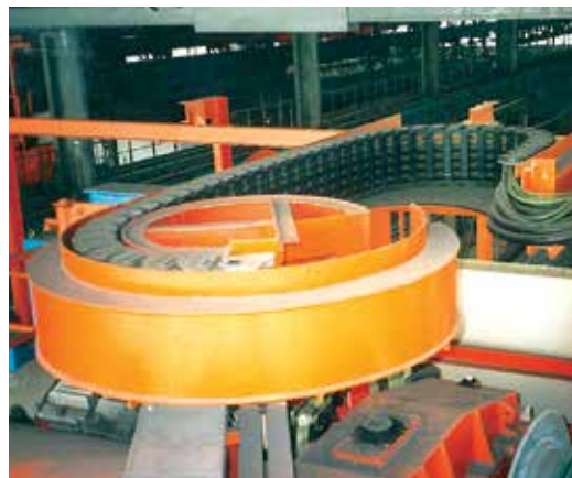
Circular motion of 180° with standard e-chain® on a crane turret drive
