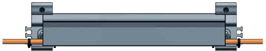
Version 01 - short trough bracket Part No. GF9.2.12 with integrated strain relief, possible ± .20" (5 mm) vertical adjustment
