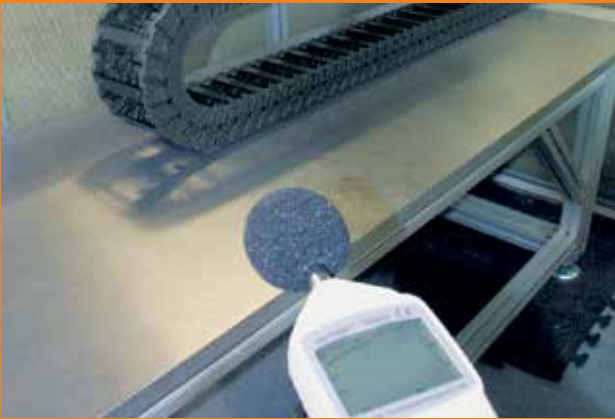
Noise level test inside an igus® acoustic cell
