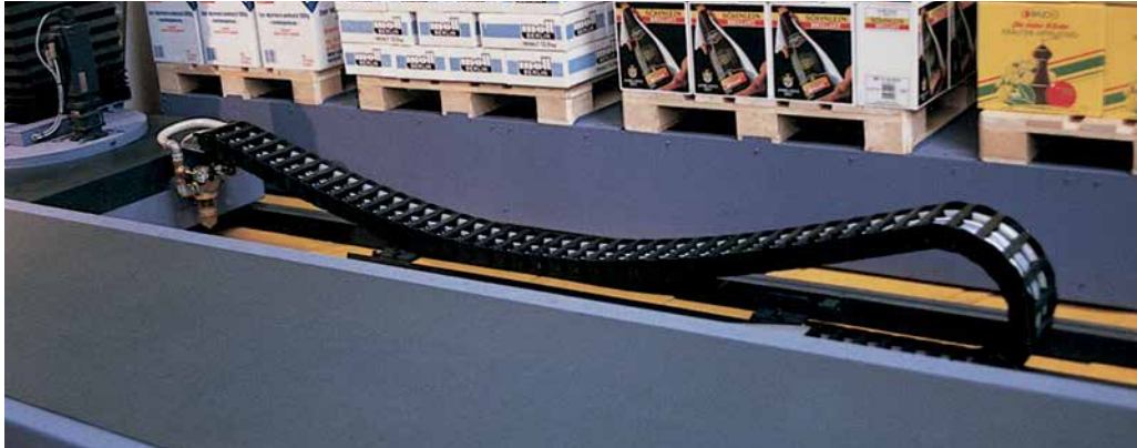
Example of unsupported with FL B sag
