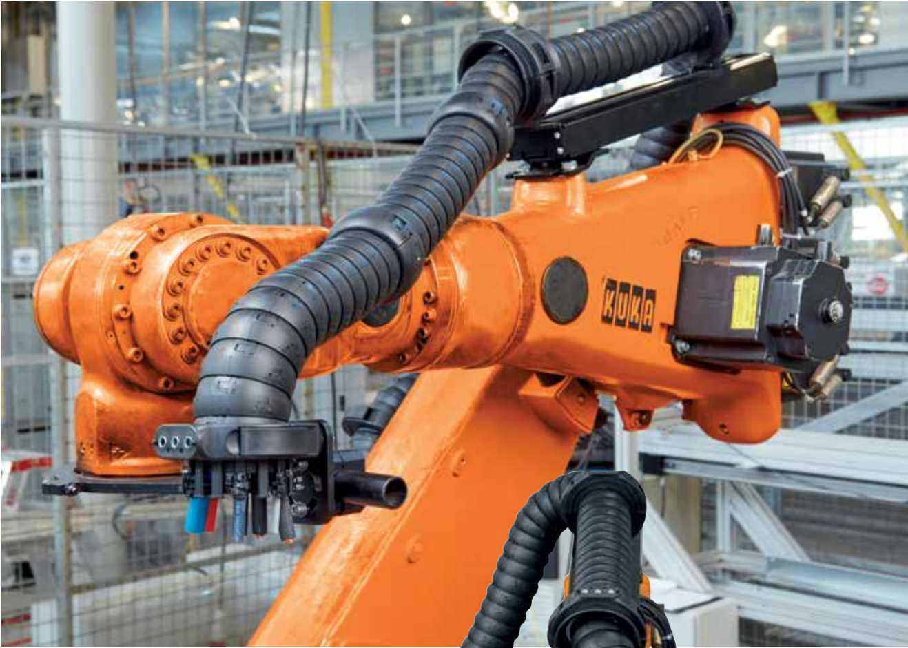
triflex® RSEL - cost-effective and space-saving guidance of the e-chain®
