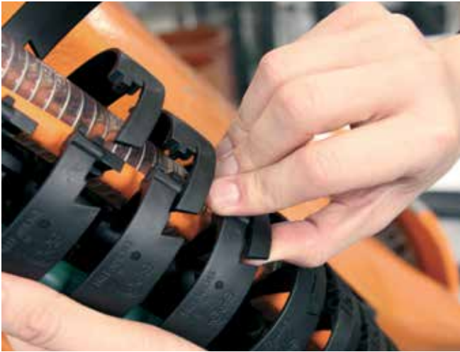
igus® triflex® R TRLF - light version, easily openable by hand or with a screwdriver
