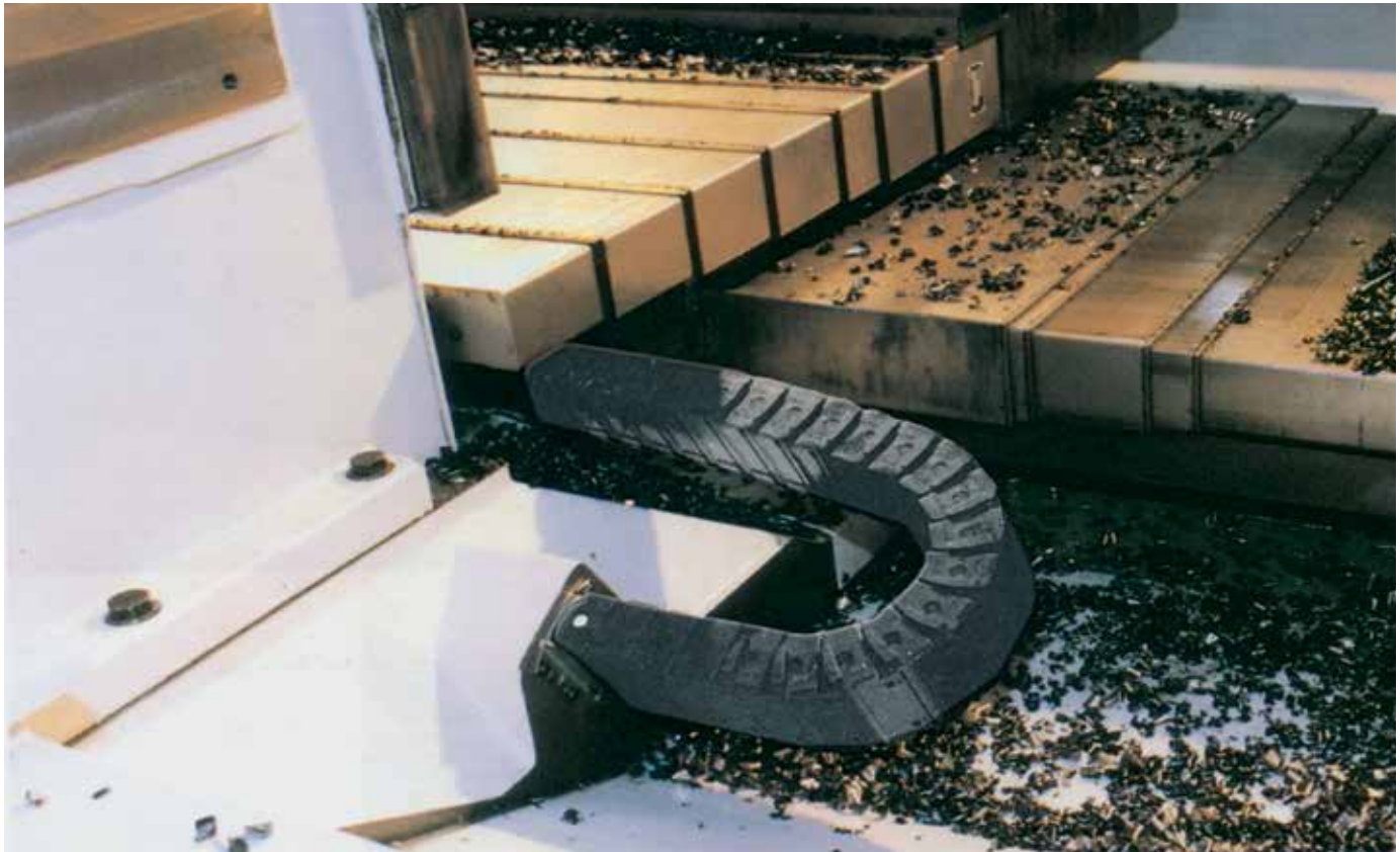
E2 e-tubes in chip area of a machine tool. Resistant to chips up to +1,562°F with special igumid HT material
