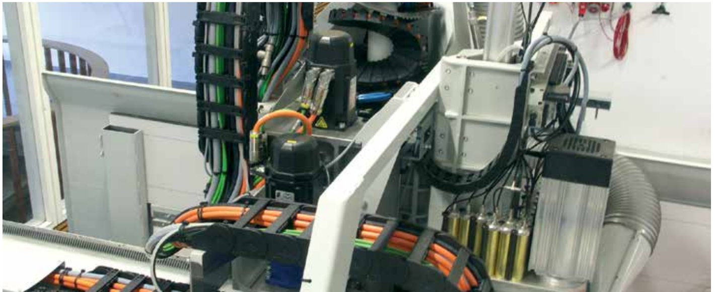
igus® twisterband and other e-chains® in a wood working machine
