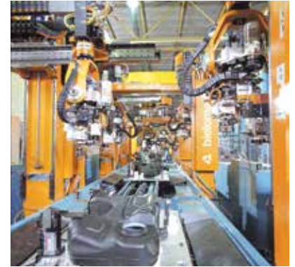
Multi-axis E-Chains® E-Z triflex® on a production line, combined movements
