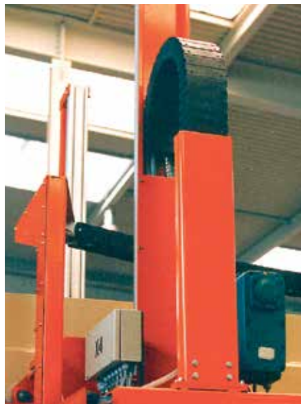
Standing application with support of the first chain links; R68 e-tube
