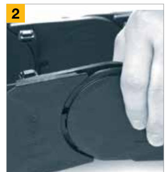
2 Insert screwdriver into the slot between the side links. Using a lever action, release the side links
