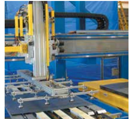
Series E6-52 high speed 49.2 ft/s (15 m/s) low noise operation, optimized noise level
