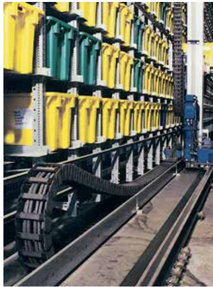
Automated storage/retrieval system with System E2 and chainflex® cables - travels up to 262 ft (80 m) and speed of 14.8 ft/s (4.5 m/s)
