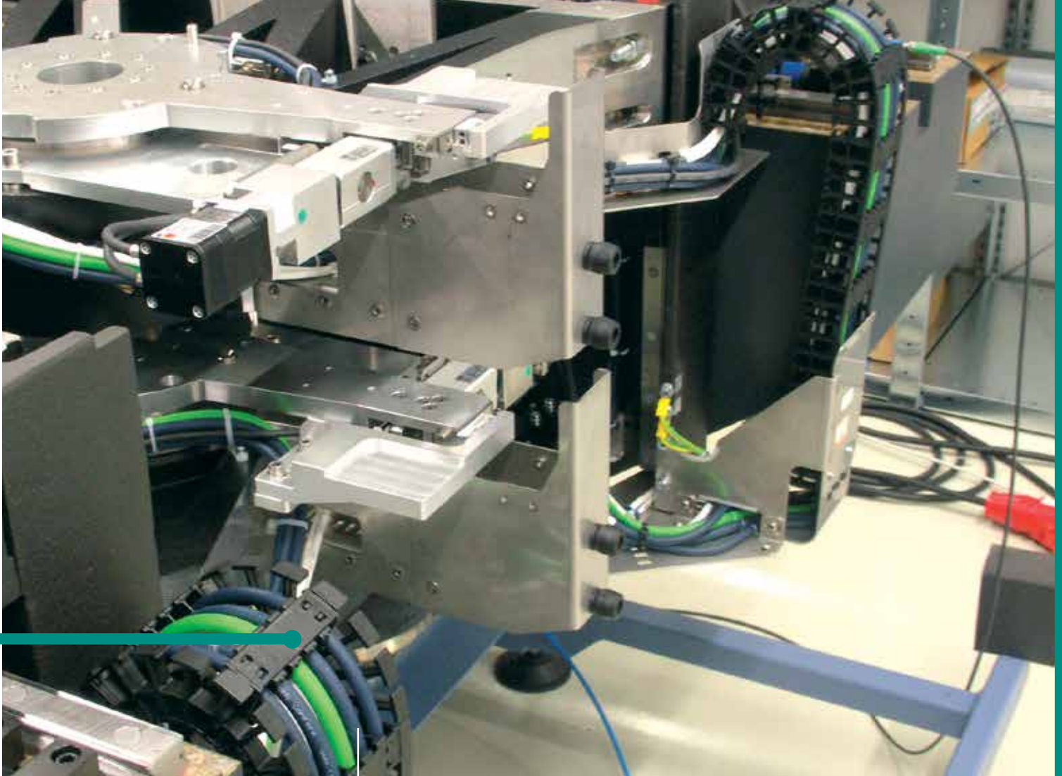
T3 system on the Z-axis in the positioning system. It has very low vibration and is quiet.
