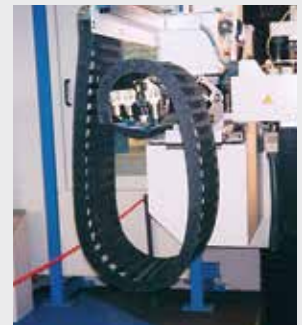
Vertical rotary motion of an E2 e-chain®
