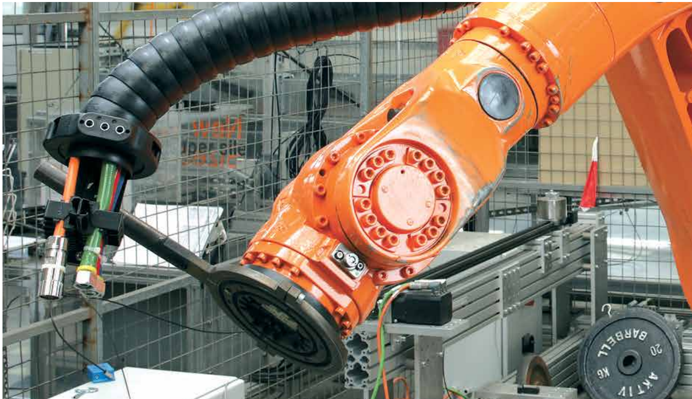
Individual strain relief for every cable offers security and easy replacement
