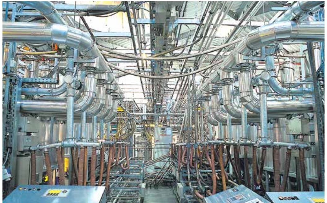
igus® factory; automatic compounding and conveyor belt for igumid G
