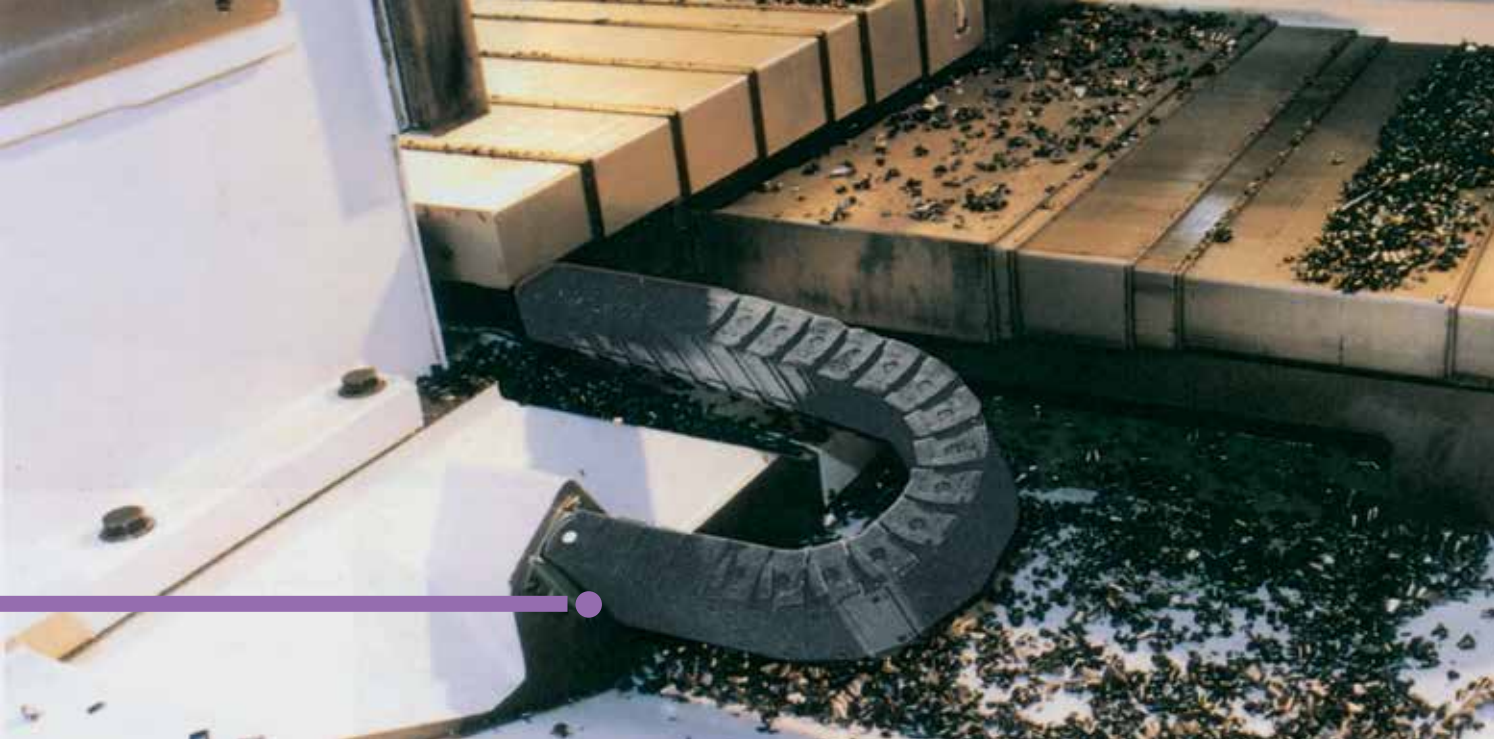
E2 e-tubes in chip-area of a tooling machine. Resistant against hot metal chips up to 1,562°F (850°C)
