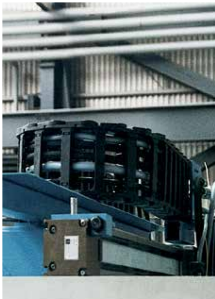
e-chain®, side-mounted, supported System E4
