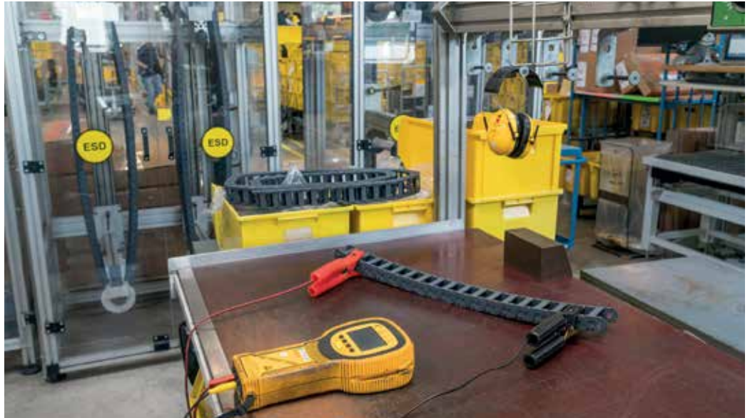
100% of the produced ESD e-chains® are checked for their continuous conductivity from one end to the other
