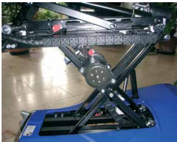
Series E1-17-021-028 in an electric wheelchair - cable supply on the scissor lifting system
