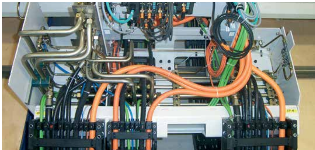
Chainfix strain relief with KMA brackets; used here for cables and hoses
