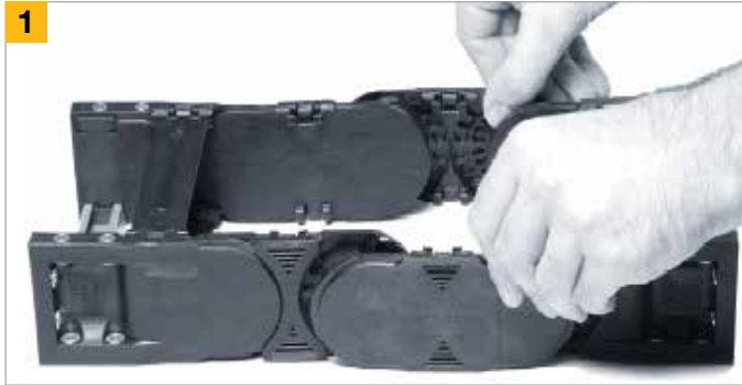
1 Line up the two inner side links, side by side
