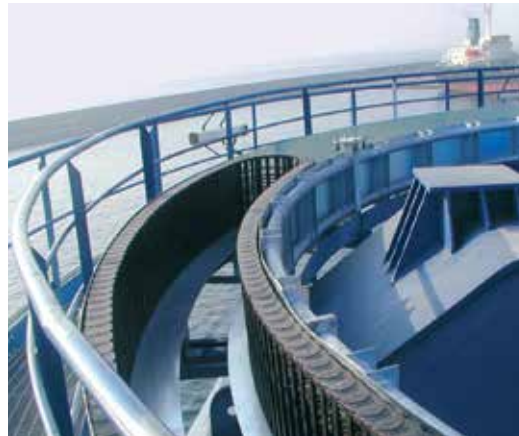
RBR-rotary movement with igus® System E4, installed on a crane
