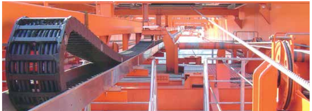
Long travel with E4 rol e-chain®, guided in a igus® steel guide trough
