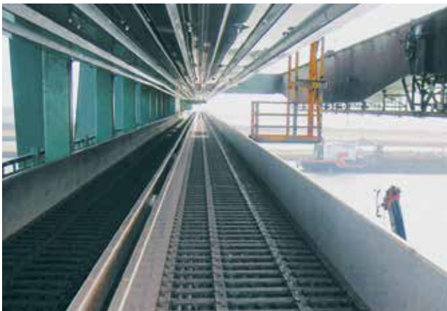
igus® System E4 with extension link at a ship loader for the coal unloading. Travel 344.5 ft.(105 m), speed 787 ft/min (240 m/min), load 35.6 lbs/ft (53 kg/m)
