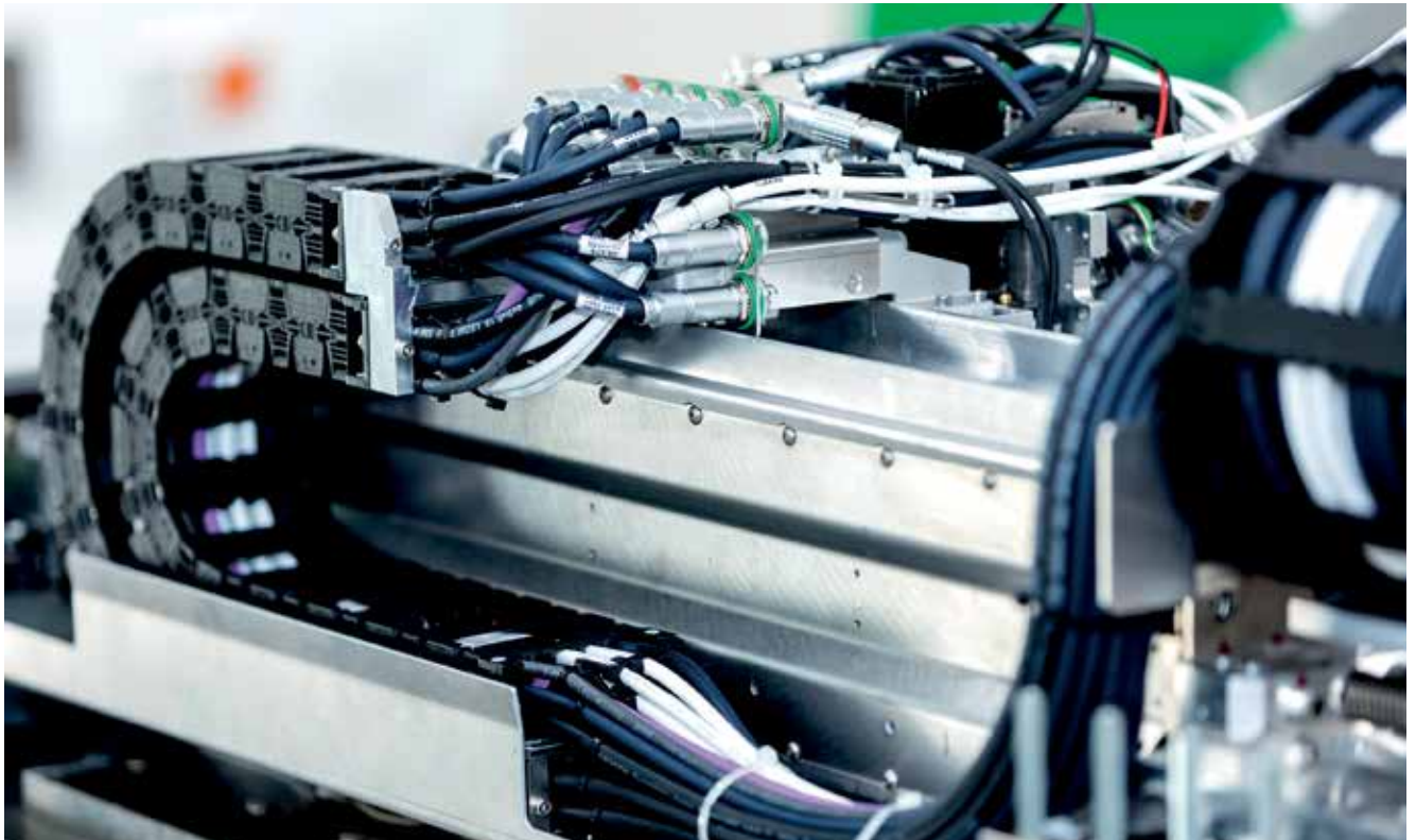
Cleanroom suitable E6-1 series as harnessing readychain® system for a semiconductor industry
