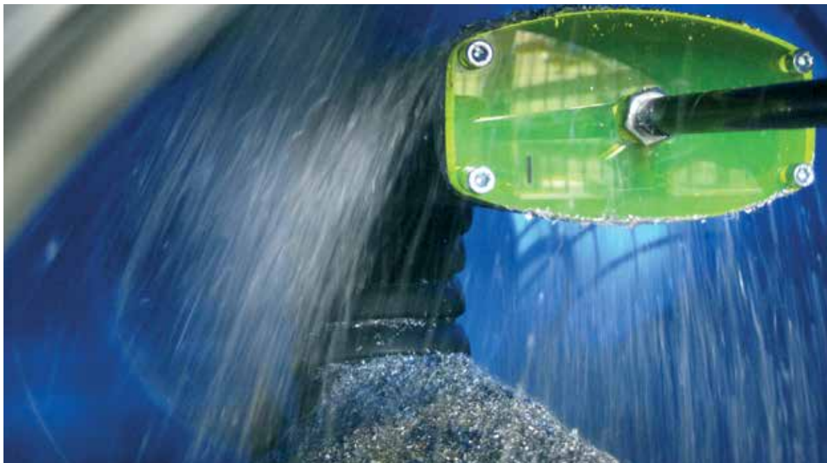
Chip-test at the igus® test-lab proven enormous tightness.
