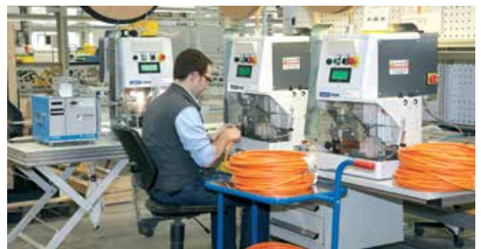
Modern machinery - automatic stripper-crimper
