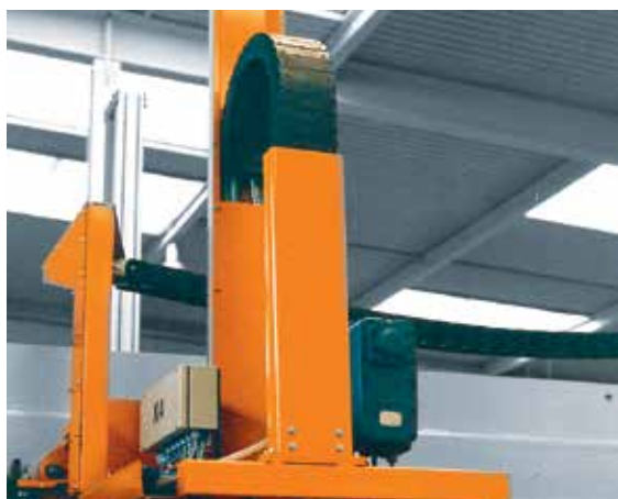
U-shaped supported e-tube for high lateral acceleration
