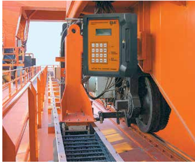
Electronic pull-push force monitor with the igus® PPDS system
