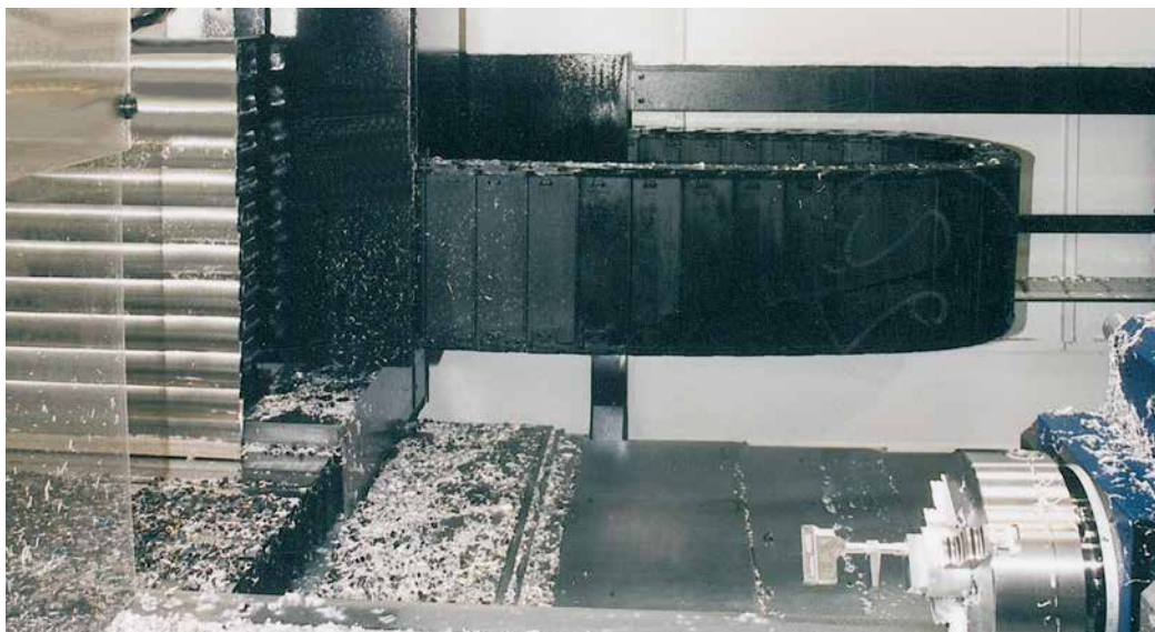
System E4 e-tube in direct chip area E4/light
