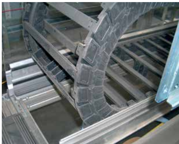
Fixed-end module - Simple fastening of the e-chain® without drilling
