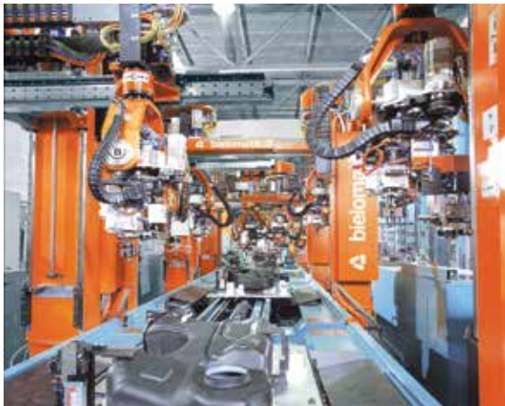
E-Z triflex® e-chains® for multi-dimensional movements on a production line
