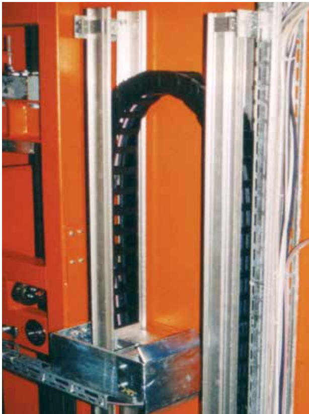
e-chain® on the tower of the storage and retrieval unit for high-bay warehouses rolls off from one aluminum guide trough to the opposite one
