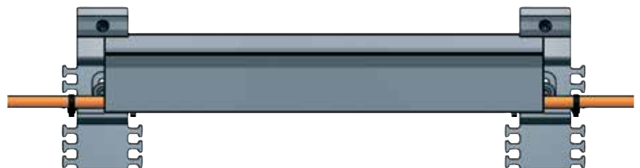
Version 02 - long trough bracket Part No. GF9-2-11 with integrated strain relief, possible ± .20" (5 mm) vertical adjustment
