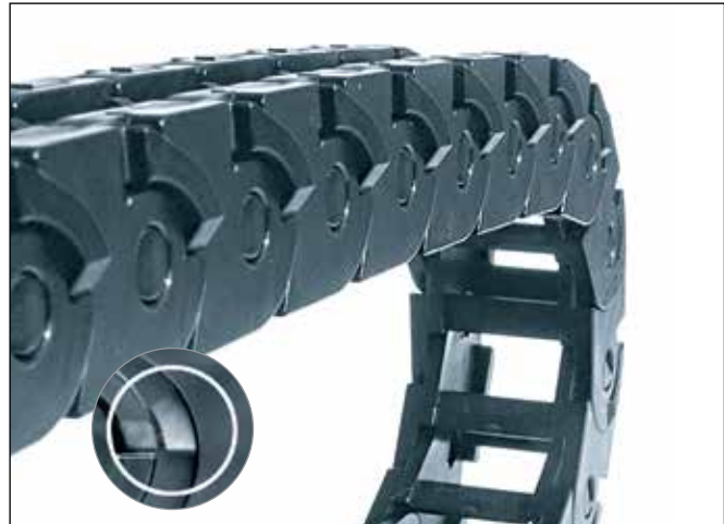
In the extended position, the wings fold out and safely hold the upper run in the elevated position
