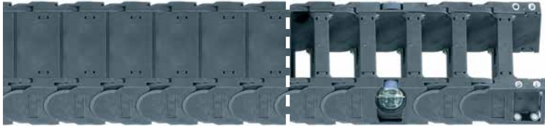
Series 4040R - crossbars every link, openable along both radii Series 8840R - fully enclosed, hinged, snap-open removable lids
