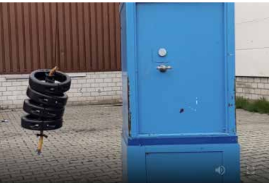
Picture 9 The testing to which the e-loop® was subjected prior to launch included break tests involving impact on a steel safe.
