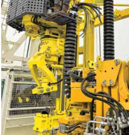
Picture 1 Service loops used to be the standard solution to supply energy to top drive drilling rigs.
