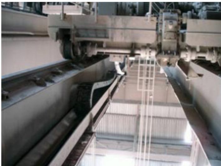
The same two-girder crane as above but after it has been modernized with a plastic e-chain® in an aluminum guide trough.
