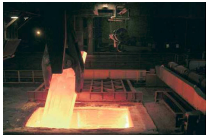
Mechanical claw on a slab crane directly above a furnace
