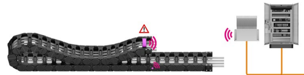
Predictive maintenance uses sensors, software and the elements of condition monitoring to create a system that allows dynamic service life calculation and determines the best times for the maintenance of igus® products. Source: igus® GmbH
