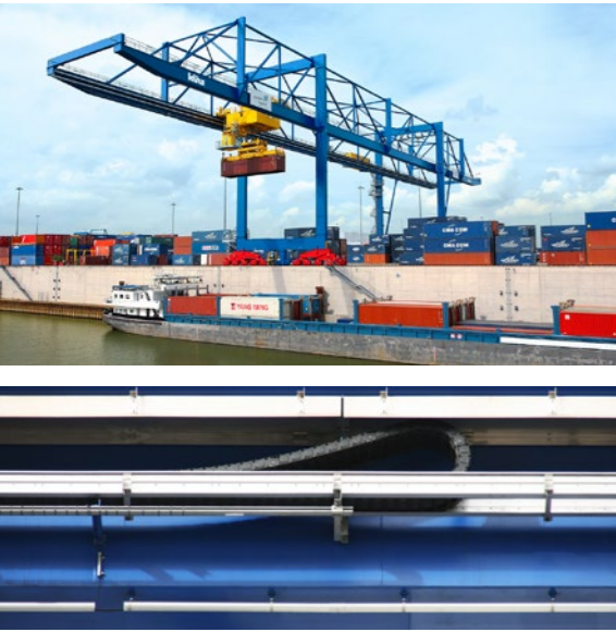
2008 – The innovation: the distributed P4 rol e-chain® has been added to the rol e-chain® product range for applications involving very high speeds (more than 240m/min) and installations where noise is very important. In use: worldwide in STS crane systems, ASC cranes, etc. Source: igus® GmbH
