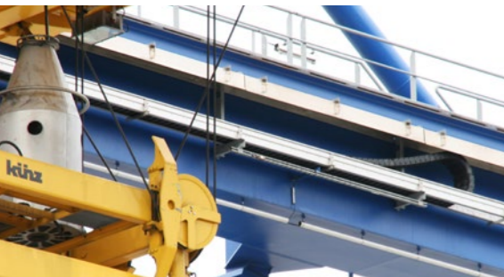
Roller energy chains are safe and compact and require very little maintenance; their cable lengths are up to 50% less than those used in festoons. Source: igus® GmbH
