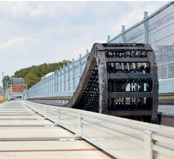
Energy chain systems are tested at speeds of up to 8m/s over a travel of 400 metres. You can see the test system in the video below: https://youtu.be/QusrqQ41ZEw Source: igus® GmbH
