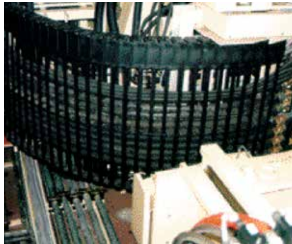
Hydraulics and electric cables are separated from one another in this example
