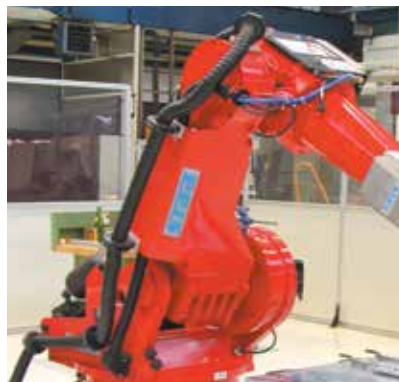
Complex movements with igus® triflex® R, combined movements
