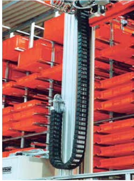
The E4-1 system is one of igus® best solutions for hanging applications
