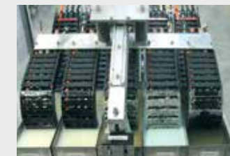
igus® tests: e-chains® and chainflex® cables are tested for resistance against chemicals and oils in long-term tests
