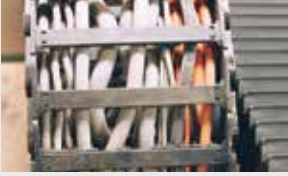
Corkscrewing: an effect of improper cable and hose placement in an e-chain®
