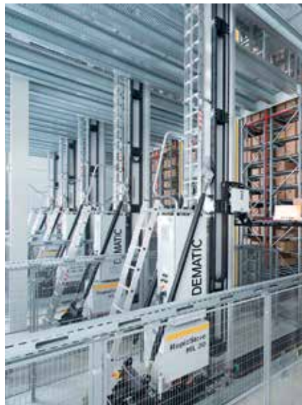
igus® guidelok slimline P vertical guidance in a high-bay warehouse
