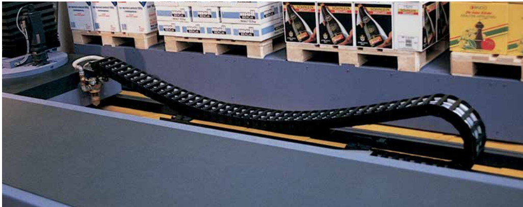
Example of unsupported with FL B sag
