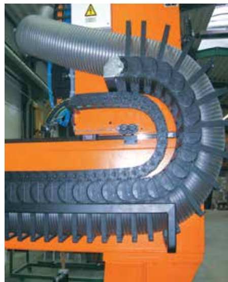
e-chain ® with extension links supports a smaller e-chain ® with electric cables
