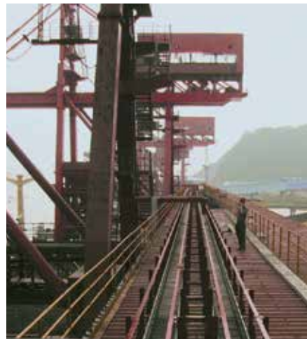
Series 4040R rol e-chain® on a coal unloading system - travel 623 ft. (190 m), speed 1.64 ft/s (0.5 m/s), fill weight 5.41 lbs/ft. (8.05 kg/m)
