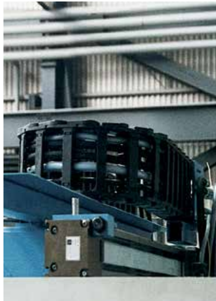
e-chain®, side-mounted, supported System E4
