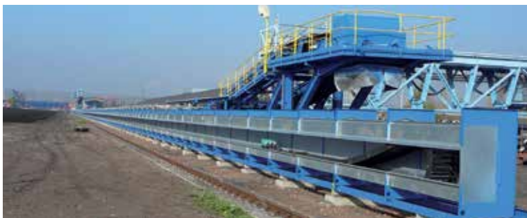
Longest igus® travel of 2,018 ft (615 m) with rol-e-chain and chainflex® cables
