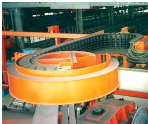
Circular motion of 180° with standard e-chain® on a crane turret drive
