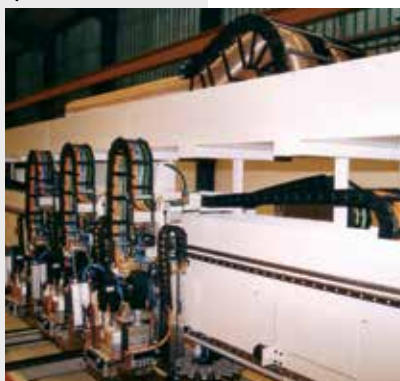
Extension links for E2 and E4 for large conduits, cable and hoses
