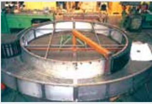
Rotary motion with RBR , diameter 236.2" (6,000 mm), with RBR the inner ring rotates
