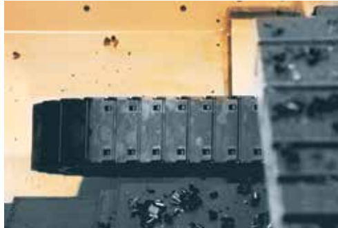
igus® e-tubes in the chip area of machine tools
