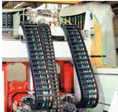
readyChain® with combined motions on tooling machines
