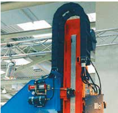
Vertical, standing Series E4/light, up to 19.69 ft (6 m) possible
