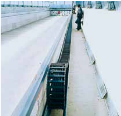
Gliding application System E4, up to 1641 ft (500 m) realized
