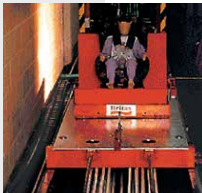
Crash test unit: 72.2 ft/s (22 m/s) speed and 2,572 ft/s 2 (784 m/s 2 ) acceleration, travel speed
