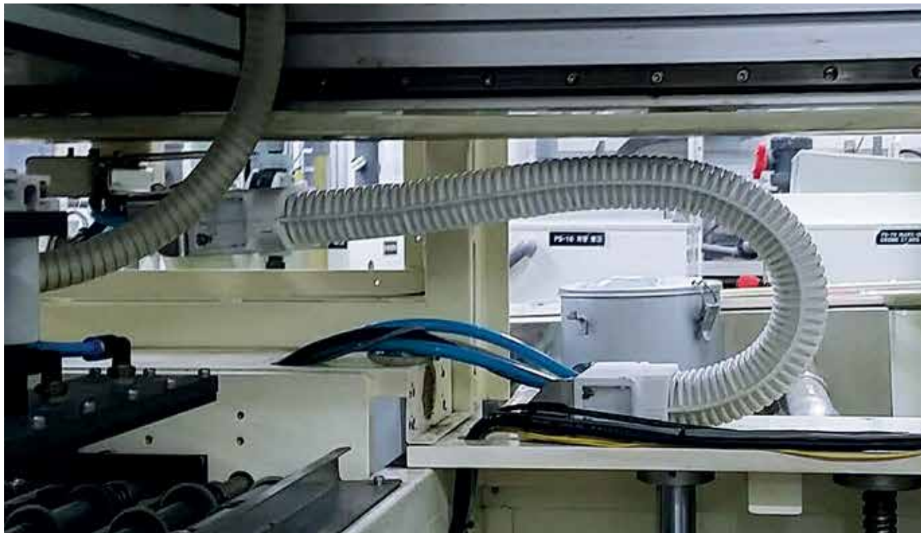
Absolutely dust-free environment for printed-circuit-board production using the abrasion-resistant e-skin® from igus®
