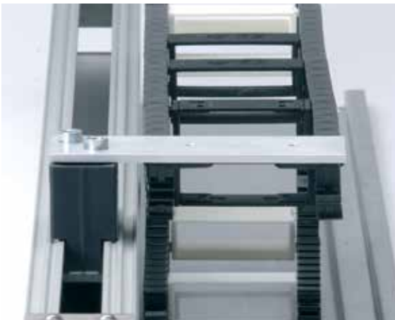
Testing facility at the igus® laboratory System T3 - ideal for high accelerations and short strokes
