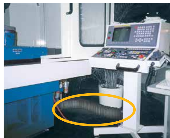
triflex® 332 as unsupported link from machines to control desk
