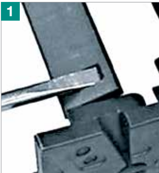
1 Lever crossbars with screwdriver
