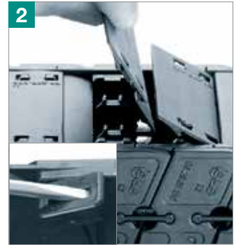
2 ... and remove lids by hand
