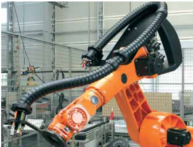
triflex® RS for a low profile retraction system.. Integrated fiber rods generate the directed pretension so that loops do not form in the working area
