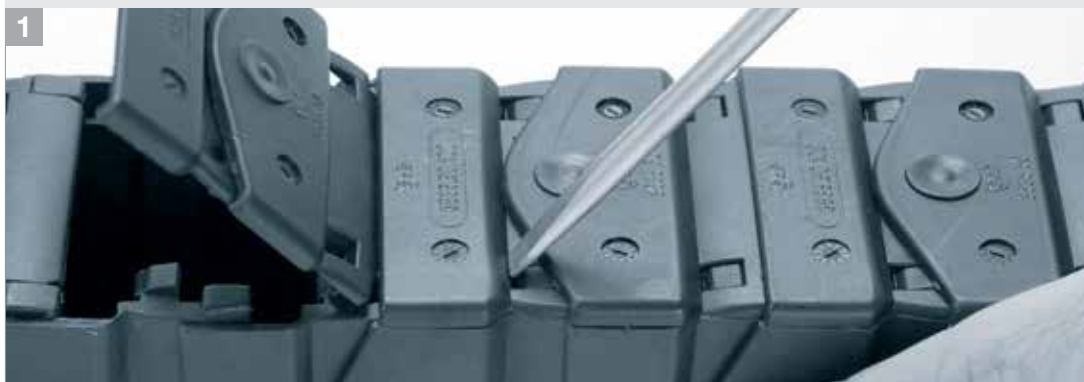
To open Series 352 and Series 353 only - Insert screwdriver into slot on top of lid and push down
