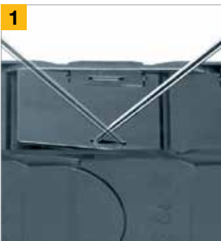
1 Remove lids/bottoms - Insert screwdriver into the slot, using a lever action apply pressure to the screwdriver to release
