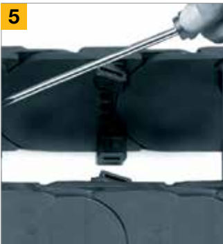
5 Assemble clips (for e-chains with crossbars every other link) - push down and snap in using a screwdriver
