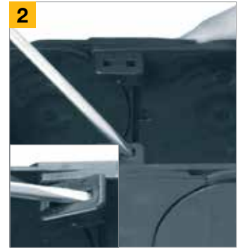
2 Remove clips - Insert screwdriver into the slot, using a lever action, apply pressure to the screwdriver to remove the clip
