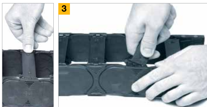
3 Snap the crossbars into place
