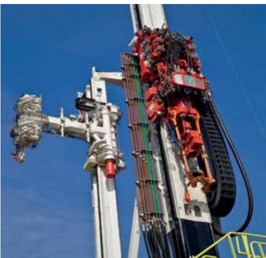
Compact design, custom configuration: two nested E4-112 e-chains® each around 39.4 ft. (12m) long carry very heavy fill weights
