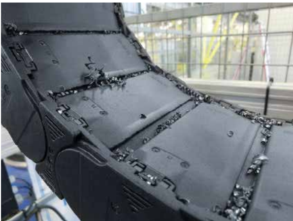
Denseness test at the igus® lab: High chip protection in the test. Stop-dogs completely free of xhips
