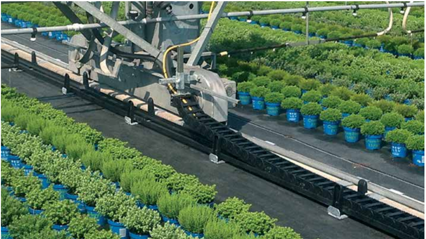
E2/000 Rol e-chain® in a Guidelite guide trough of an irrigation plant
