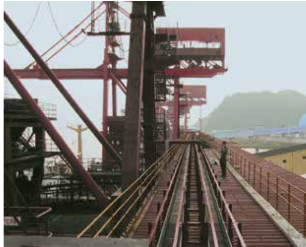
Series 4040R on a coal unloading system - Travel 623 ft. (190 m), Speed 1.6 ft/s (0.5 m/s), Fill weight 5.41 lbs/ft (8.05 kg/m)
