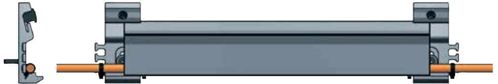
Version 01 - short trough bracket Part No. GF9.2.12 with integrated strain relief, possible \pm .20^\circ (5 mm) vertical adjustment
