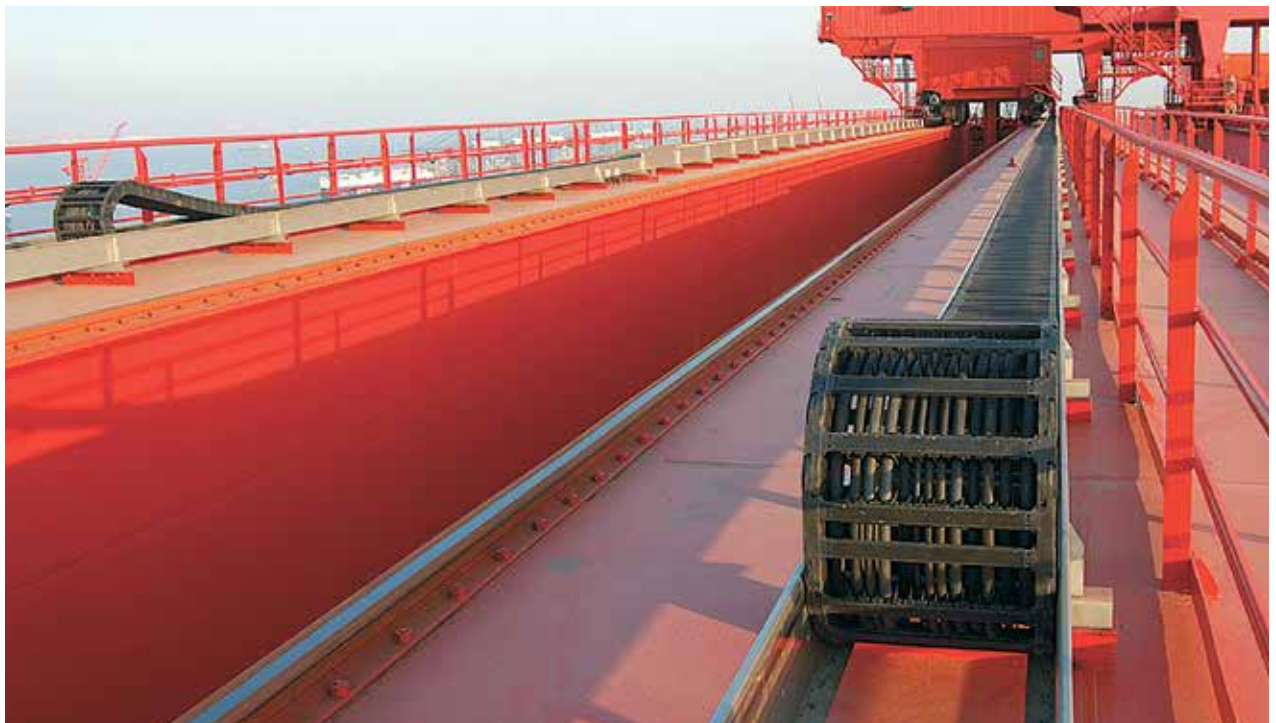
Shipyard-Crane: 590.5 ft. (180 m) travel, 20.16 lbs/ft (30 kg/m) fill weight: No problems since installation in 2001 with igus® rol e-chain®
