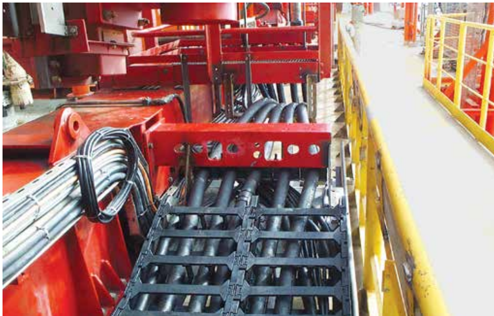
Lightweight and high stability: igus® e-chain® tames stiff hydraulic hoses
