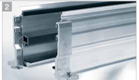
1 Pre-assemble heavy duty bracket and screw set 2 Fasten Heavy Duty assembly set outside. Please note: half the length of the assembly set and connector must protrude out of the trough.
