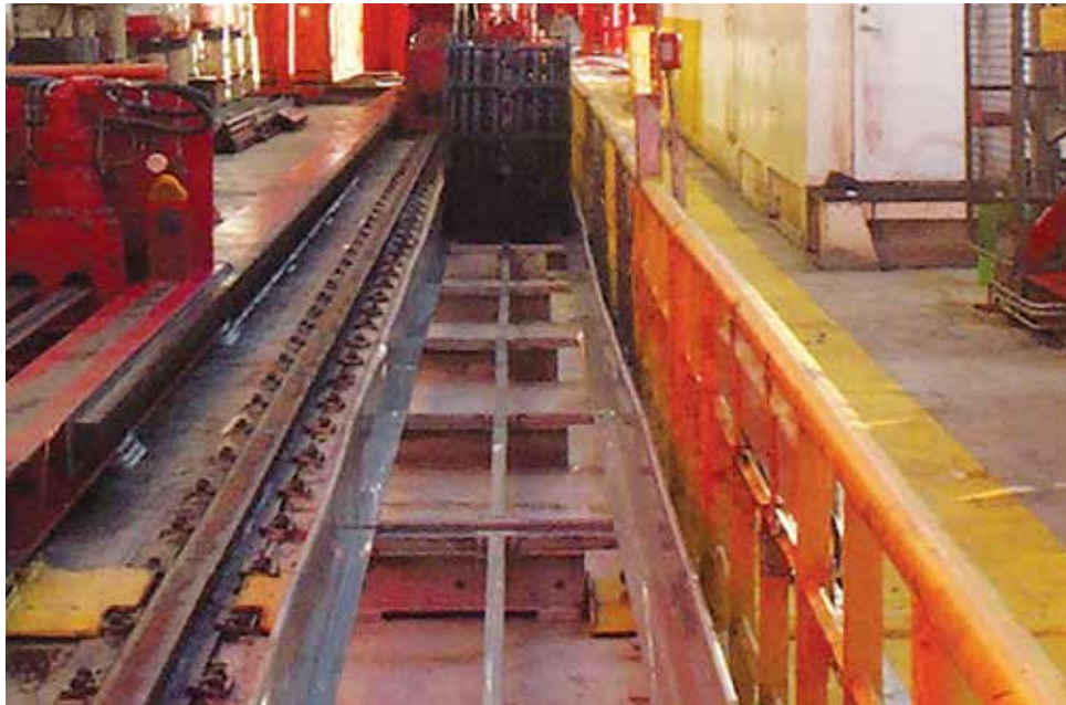
System E4 with extension links, long travel application on board West Navigator (Norway)
