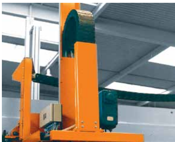
U-shaped supported e-tube for high lateral acceleration
