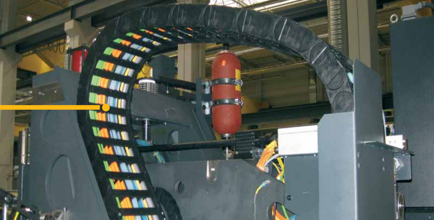
The E4-42 series in a machine tool, completely assembled with igus® chainflex® cables
