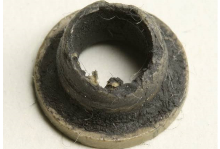
High speed rotation caused overheating, which led to lost press fit and the bearing rotating in the housing instead of the shaft. Dust originates from the housing and bearing material.
