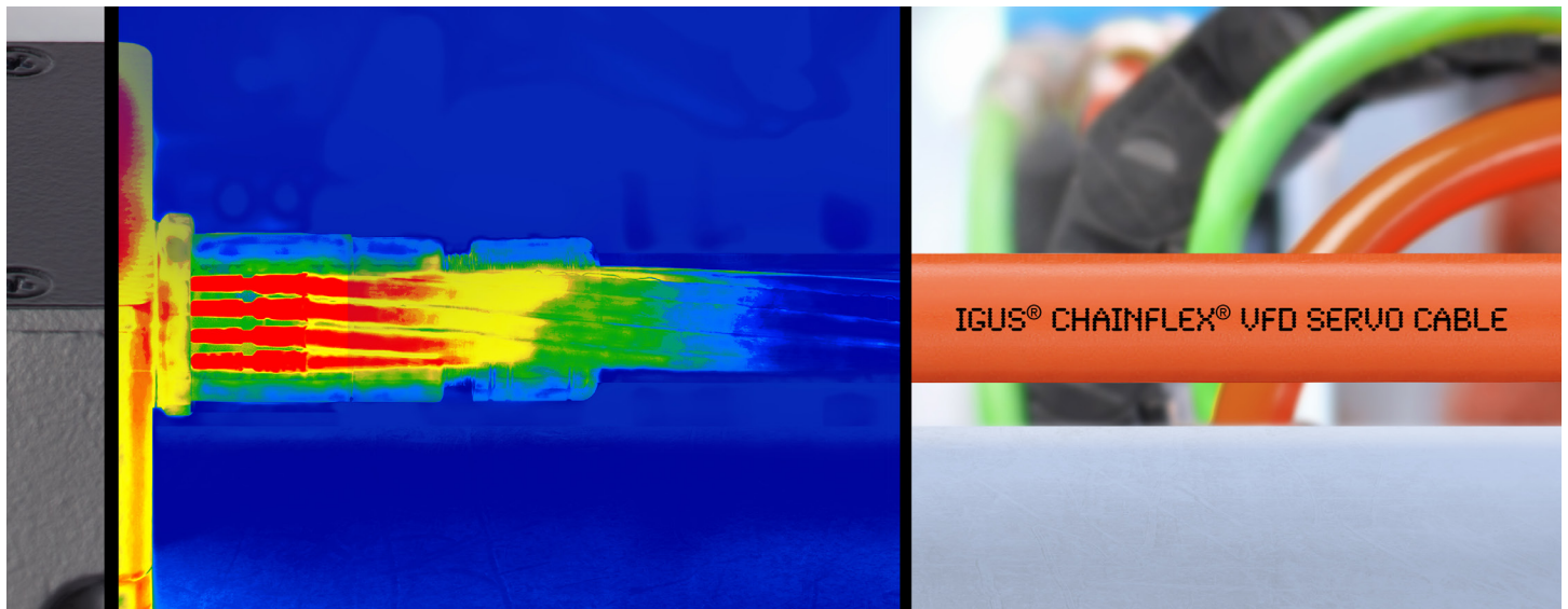
Test shows heat propagating into the cable
