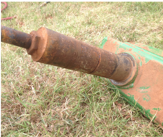
Result of using a thin, ineffective corrosion inhibitor on a shaft after only one season
