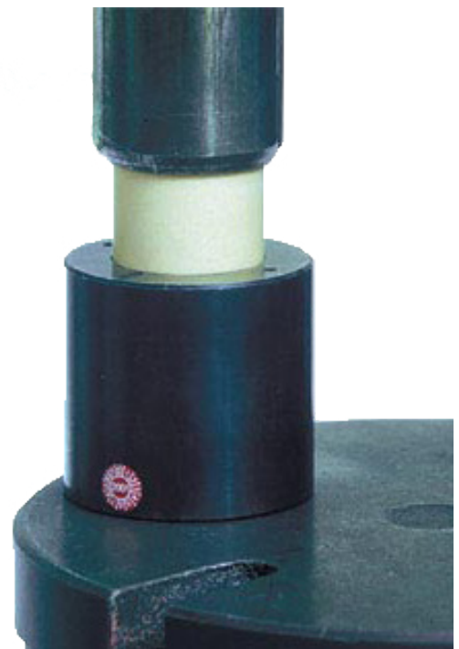
arbor press used to press-fit a plain bearing during installation
