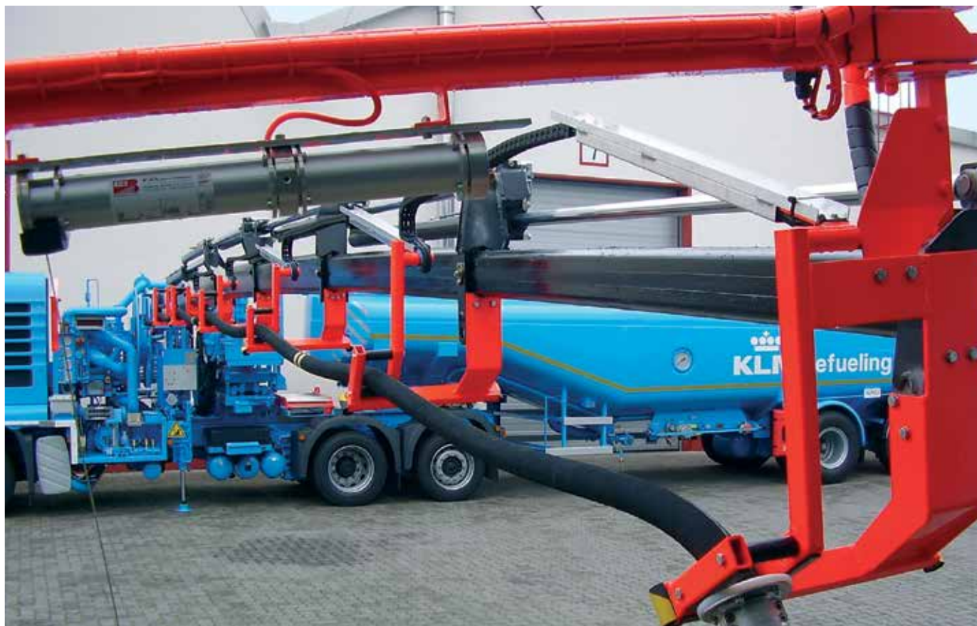
E2/000 series 1400 in aircraft refueling truck - telescopic crane with six sections
