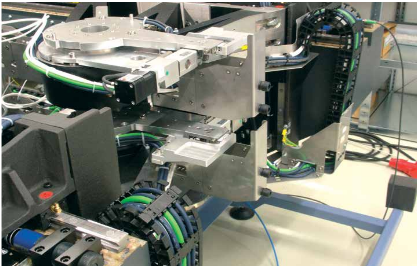
T3 system on the Z-axis of a positioning system. It has very low noise and vibration
