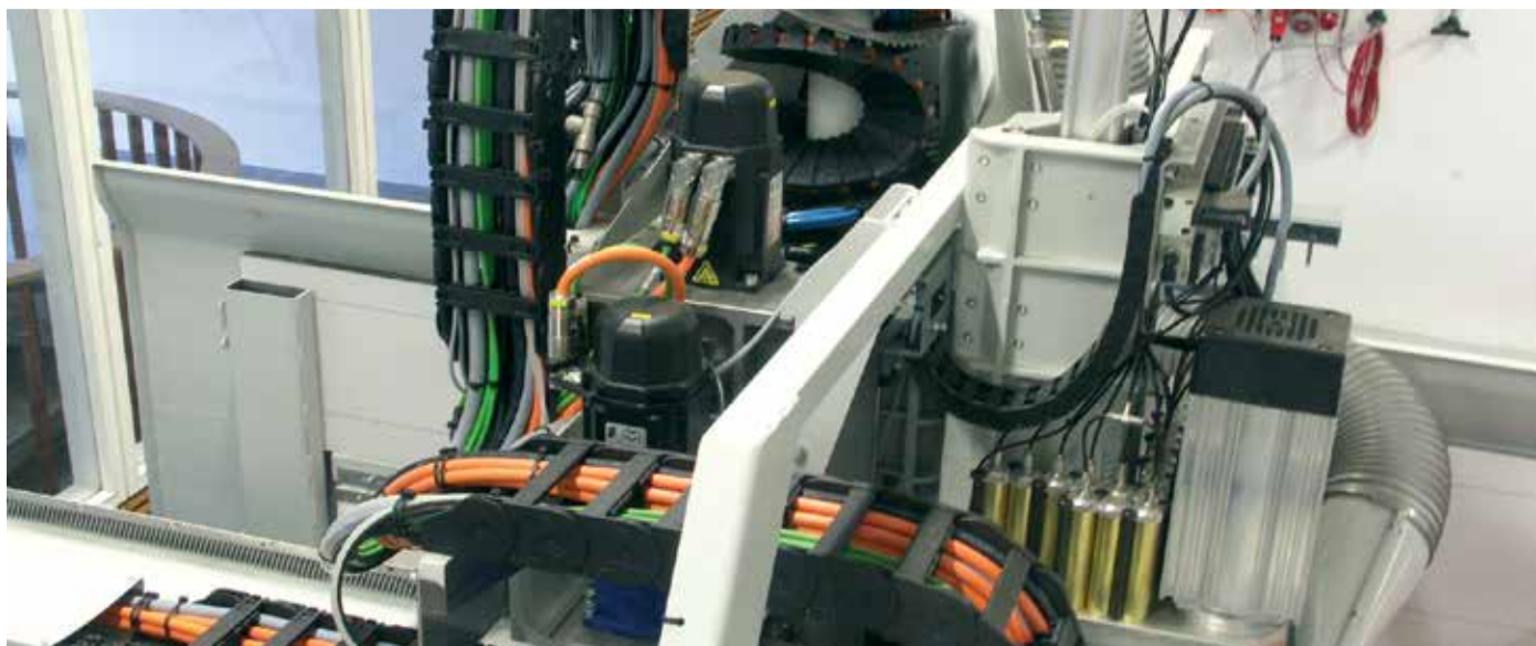
igus® twisterband and other e-chains® in a wood working machine
