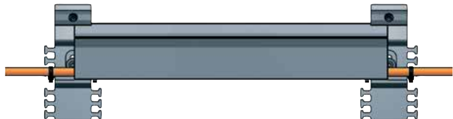
Version 02 - long trough bracket Part No. GF9.2.11 with integrated strain relief, ± 5mm vertical adjustment (electrically conductive version: GF9.2.11.CD)
