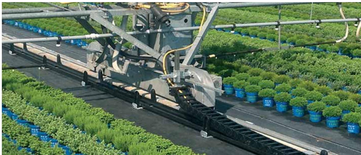
E2/000 rol e-chain® in a guidelite guide trough on an irrigation plant
