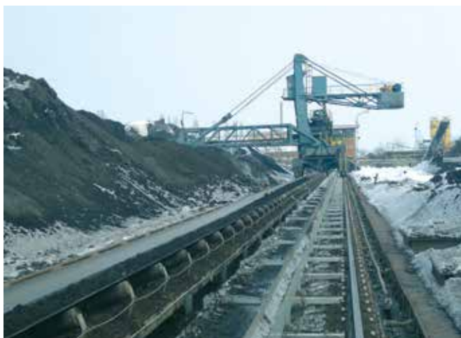
Series 4040HD on 591ft (180m) travel lengths with housing. Temperature range from -40°C/+40°C and in very dirty environments
