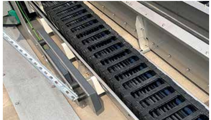
P4.1 e-chain® with EC.PP in the igus® outdoor test
