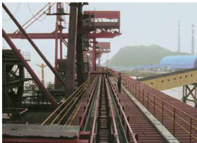
Series 4040R on a coal unloading system. Travel 623ft (190m), speed 1.645ft/s (0.5m/s), fill weight 5.41lbs/ft (8.05kg/m)
