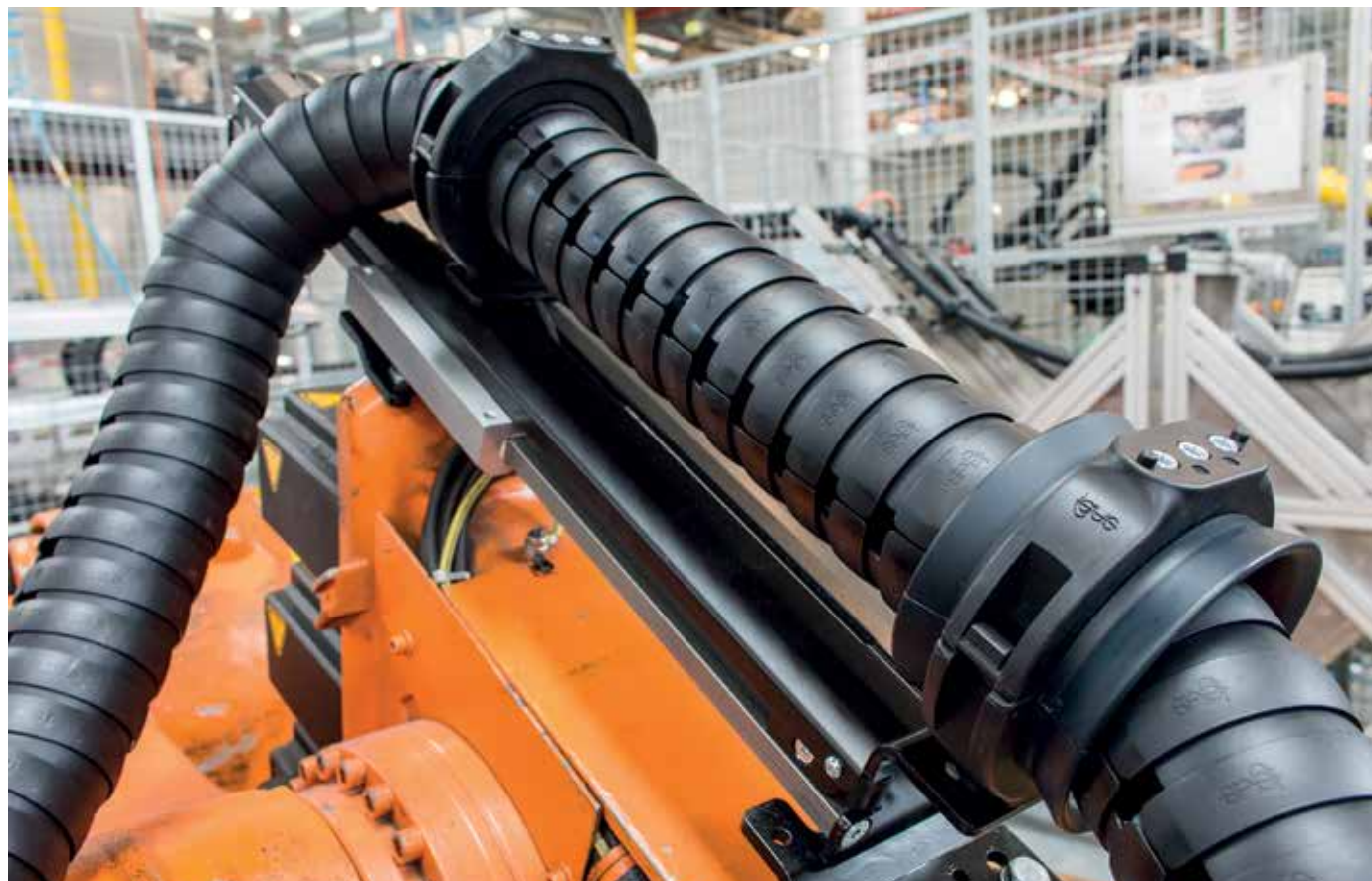
igus® TR.RSE system on test robot
