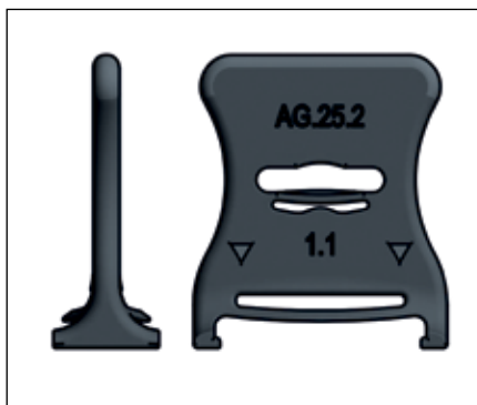
Special autoglide 5 separator available for 2400AG5 series
