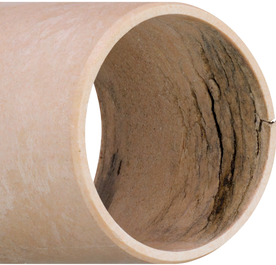
Damage due to permanent overload (Source: igus®)
