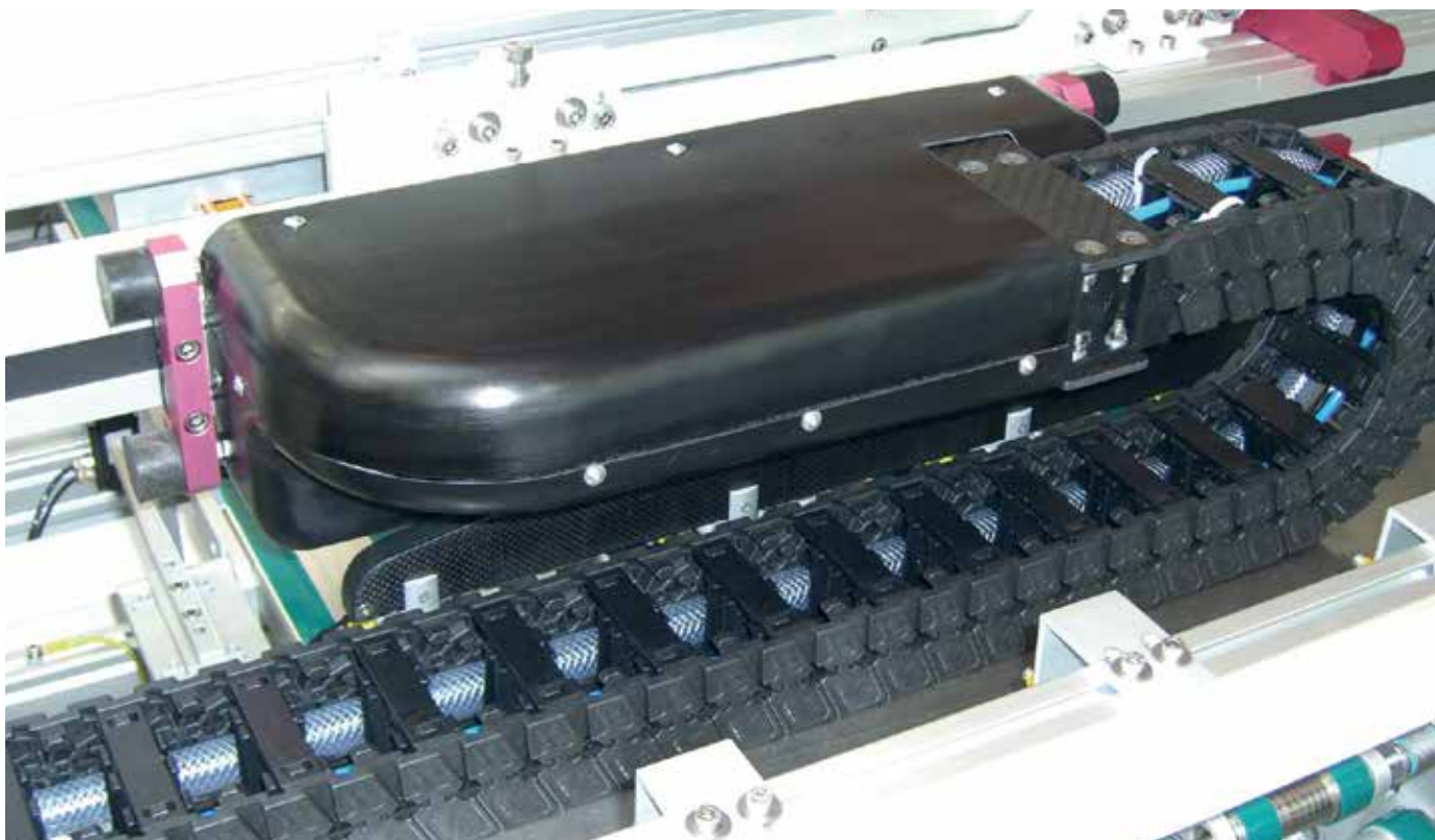
igus® system E6 guiding an extraction hose - speed 26.25 ft/s (8m/s), acceleration 257.5 ft/s 2 (78.5m/s 2 )
