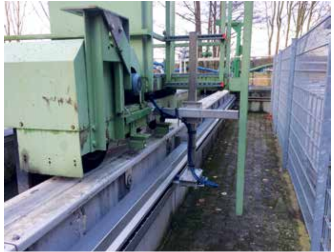
Sand trap with telescopic igus® moving end arm - travel 62.34 ft (19m)
