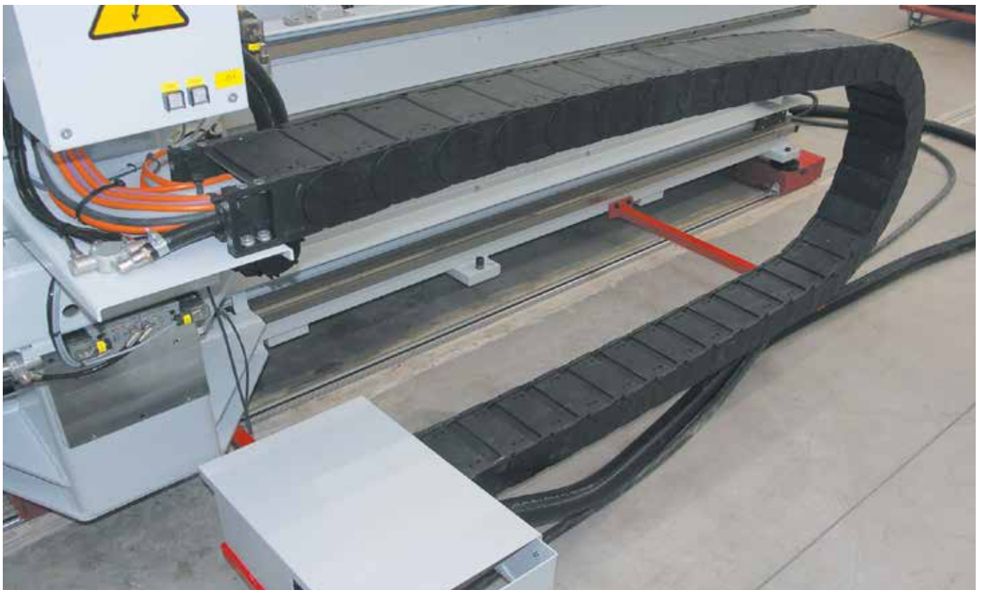
E4/light e-tubes protect cables and hoses against dirt and chips
