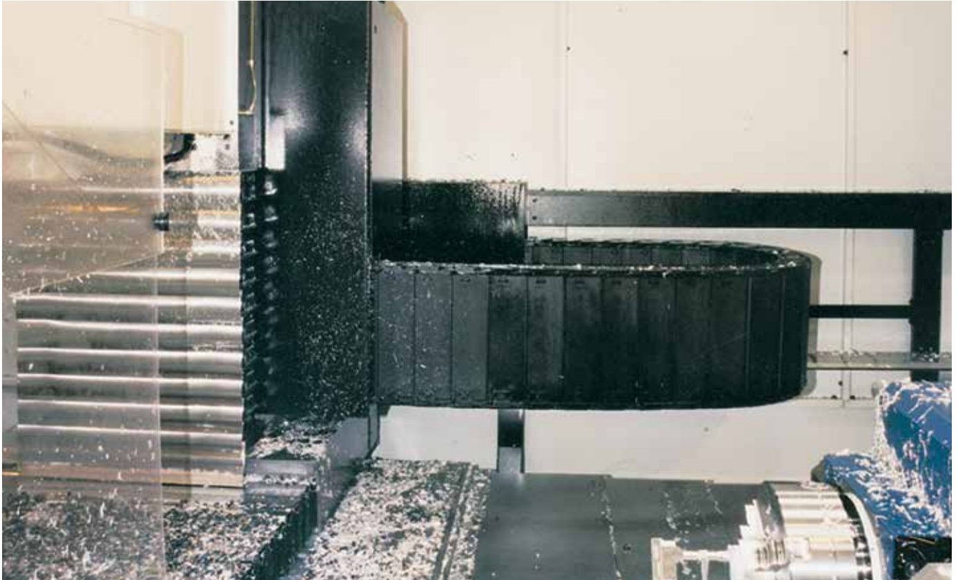
Side-mounted E4/light e-tubes - machine tool fitted with a chip-repellent e-tube from the E4 modular system
