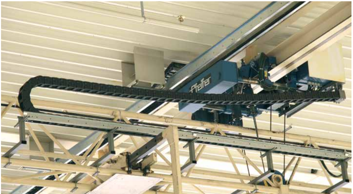
Handling unit indoor crane - long unsupported span with an igus® E4 series
