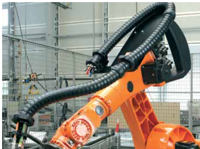
triflex® RS for a low profile retraction system. Integrated fiber rods generate the directed pretension so that loops do not form in the working area
