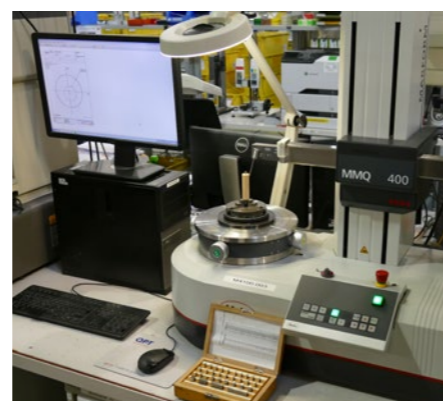
Measuring of the inner diameter of a press-fitted bearing
